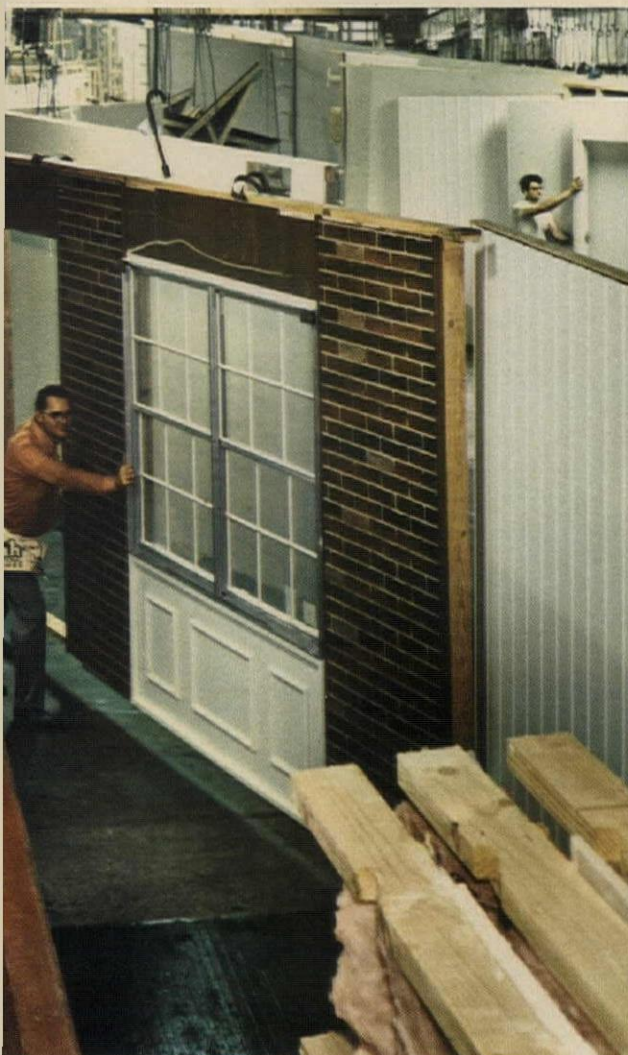
Factory assembly of prefinished aluminum products into home modules is done with ease in National Homes plants.
