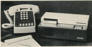
Automatic answering system answers the telephone and gives the caller a prerecorded message which can run from 20 sec. to 3 min. The compact unit can be connected to
