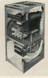
Residential-type gas furnace with heating capacities from 110,000 to 200,000 BTUHs, features a compact cabinet with a baked-on enamel finish. The unit includes a "Duracurve" heat exchanger finished in a special vitreous enamel, continuous port steel burners, a sulky mount blower and a large hammock filter. Furnace is designed so that air conditioning can be added. Lennox, Marshalltown, Iowa.
