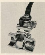
Ball valves are designed so that all internal parts can be removed and inspected without taking the valve out of the pipe line. Ball is free-floating and self-aligning. It minimizes flow resistance and can be used in limited spaces. Lunkenheimer, Cincinnati, Ohio.
