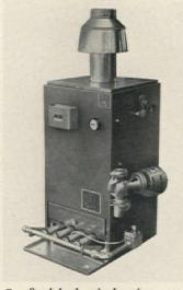
Gas-fired hydronic heating system is available in nine models ranging from 64,000 to 320,000 BTUHs. The system, engineered for long term efficiency, utilizes a fire tube design and stainless steel baffles for maximum heat transfer. All controls are conveniently located on unit exteriors. A special door provides quick, easy access to pilot and main gas burners. Columbia Boiler, Pottstown, Pa.
