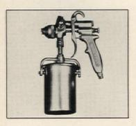
Medium production spray gun can operate from a pressurized material supply tank or be easily converted to a cup gun siphon operation. Weighing only 11/2 lbs., the gun provides high quality atomization in pattern control. Suitable for use with lacquer and enamel finishing, the unit, which works on 1-11/2 hp air supply, sells for under \$35. Spee-Flo, Houston, Tex.
