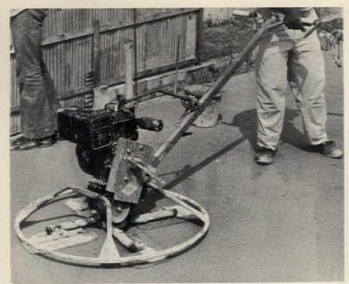
Heavy-duty 36" diameter power trowel with sliding sleeve-type clutch and a dead man lever meets OSHA standards. Tool has finish
