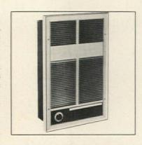
Forced-air wall heaters built for heavy-duty service are designed for large areas and for part-time occupancy areas where high-speed heat recovery is necessary. Heater features a built-in positive thermostat for automatic temperature control, and a long-life heating element. Units, which can be easily installed, range from 1.5 KW to 4 KW on 208V, 240V or 280V. Ward Leonard, Mt. Vernon, N.Y.
