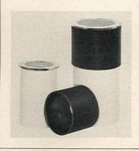
Plastic drain grates that are three and four inches in diameter have a double shoulder design that makes a snug fit inside styrene standard pipe or a coupling and fitting. It is also possible to design the drain system without couplings. Adjustments on close tolerances and dimensions are easier without the need of couplings. The grates are rustproof, resist acids and easily withstand heavy traffic wear. National Drain, Van Nuys, Calif.
