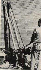
Cable puller can be adapted to use two lines for double pulling power. Tool, which can be operated by one man, pulls up, down and horizontally while standing on the floor. Weighing only 53 lbs., the puller features a telescoping shaft with 3" adjustments up to 9'. Gebo Tool & Equipment, Van Nuys, Calif. CIRCLE 255 ON READER SERVICE CARD
