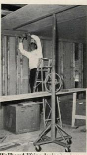
Wallboard lifting device has heavy-duty arms that lift and hold standard wallboard sections, up to 16' long, in position for seaming and nailing. Constructed of heavy steel tubing, unit has a gear drive assembly for raising and lifting and a hand wheel control. It is on wheels for easy handling. Astron, Findlay, Ohio. CIRCLE 256 ON READER SERVICE CARD
