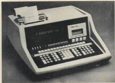
Electronic calculator features algebraic programming, making it possible to enter formulas as they are written. Instead of using standard machine language, the unit solves
