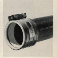
Joint fittings for use with waste piping systems eliminates the heat fusion process for connecting the piping. The only tools needed to assemble the fittings are a tape measure, a tube cutter and a torque wrench, reducing installation time. Orion Fittings, Kansas City, Mo. CIRCLE 231 ON READER SERVICE CARD
