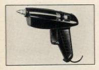
Electric glue gun has trigger mechanism that feeds solid hot-melt glue stick into unit and controls the flow of liquid glue applied to a surface. A factory set thermostat assures consistent glue melting and eliminates manual control of temperature. USM Corp., Reading, Pa. CIRCLE 251 ON READER SERVICE CARD
