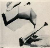
Water saver reduces up to 50% of the fresh water used in flushing standard vertical tank toilets. This saving also means a reduction of the load going into septic tanks and sewage disposal plants. The plastic device is placed in the tank and held in position by two suction darts. It channels the flow to provide the standard flushing force using only the top three or four inches of water. MVM, New York City.
