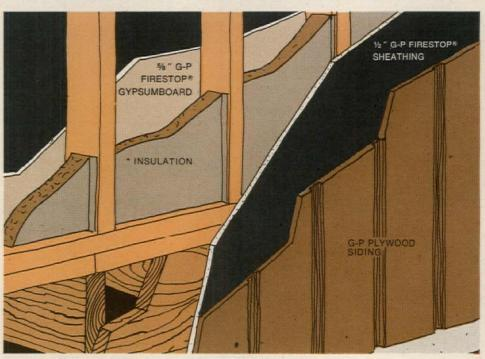
\* INSULATION NOT REQUIRED TO MEET FIRE RATINGS
