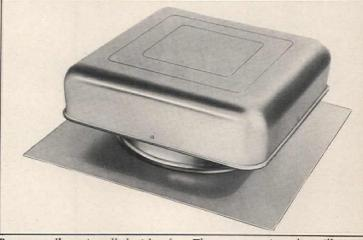
Power ventilator, installed with soffit vents, reduces attic temperature 50° or more to keep the home cooler, reduce air conditioner load and eliminate condensation problems.
