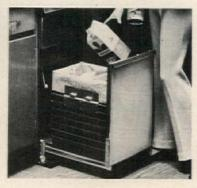
Trash compactor, into which bottles, cans and all the usual kitchen refuse may be discarded, is activated by turning a key when a full load of trash is accumulated. The compactor holds a week's worth of garbage from a family of four and includes an automatic deodorizer and disinfectant spray which works when the drawer is closed. Waste is reduced to ¼ its bulk. General Electric, Louisville, Ky. CIRCLE 273 ON READER SERVICE CARD
