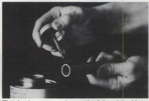
Then brush cement on the outside of the tubing. Notice how easy it is to handle. Tubing made of hi-temp Geon resists moisture, oil, corrosion, acids, alkalies and other chemicals.
