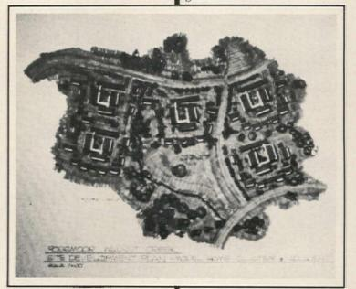
Completed plans for the initial cluster were then superimposed on adjoining areas of the project (13) to determine interrelationships of the clusters and to assure the accurate placement of buildings.
