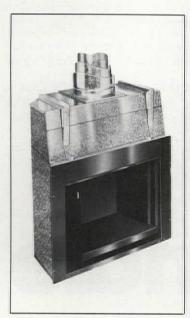
Pre-fab wood-burning fireplace system with zero clearance to combustibles has a companion masonry face and hearth set. Fireboxes have one-piece steel-reinforced cast refractories that will not break. Ashes and sparks are contained within the firebox by a special lip and an overlapping screen. Superior Fireplace, Fullerton, Calif.
