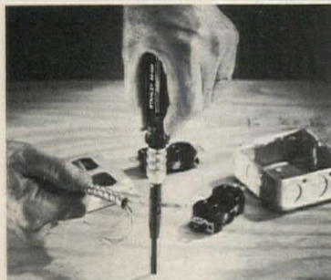
Three-in-one-tool strips insulation and cuts wire—besides driving screws.
