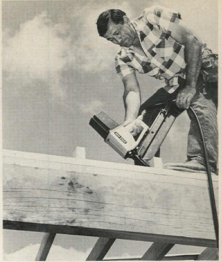
Automatic nailer can drive from 8 to 16 penny size full round-headed nails in the same magazine, which holds up to 74 nails, depending on size. Rounded nose permits tilting for flush toe-nailing. Nailer weighs 11 lbs., is 16½" long, runs on 100 to 130 psi air pressure, has a safety device that prevents it from firing accidentally. International Staple, Butler, Pa. CIRCLE 202 ON READER SERVICE CARD
