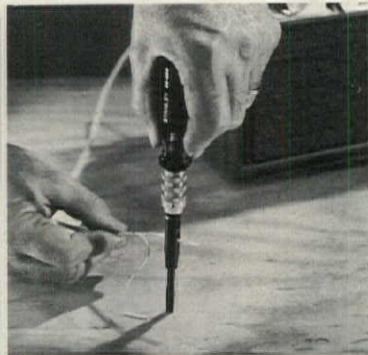
Three-in-one-tool strips insulation and cuts wire—besides driving screws.
