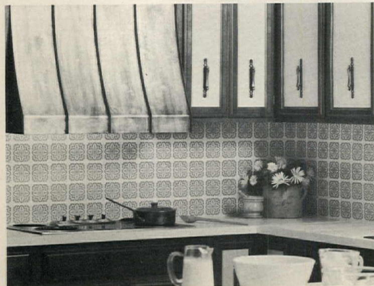
Simulated tiles are actually hardwood panels with 4" scorings. Printed on the squares is a Mediterranean tile-like design in gold, green, or blue. Then a plastic coating gives the paneling a glazed appearance, as well as protecting it from heat, moisture, and stains. "Riviera" panels are 4'x8' and 1/8" thick, can easily be cut to fit over areas like kitchen or bath counters. Also available are moldings that harmonize with the tile colors. Marlite, Dover, Ohio.
