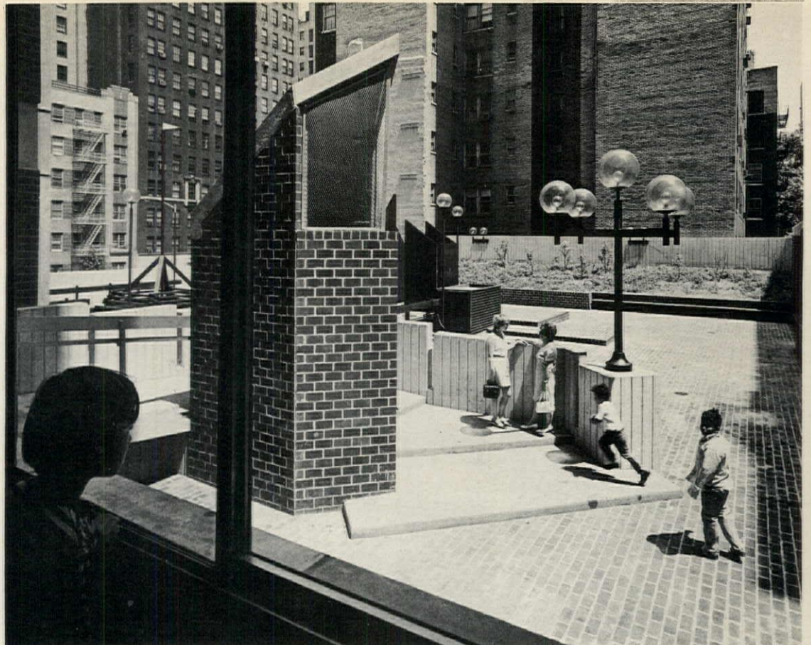
Rooftop playground activities are easily supervised through wide windows in the apartment building's second-story laundry room. Brick column, which contains air vents for garage, was designed as part of play scenery.
