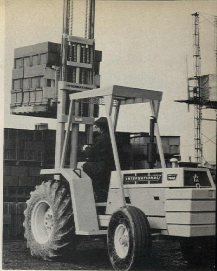
Precision handler has 14' or 17' mast that tilts 15° or 7° forward, 12° rearward, and shifts 3" right or left. It lifts to full height 5,000 or 2,500 lbs. John Deere. CIRCLE READER SERVICE 277
