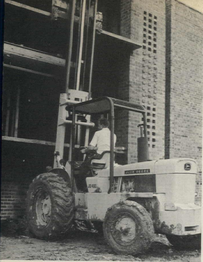
Tall-masted forklift hoists loads 28' in the air, has a capacity of 5,000 lbs. I-beam steering axle and differential lock in drive wheels offer good traction in soft ground. International Harvester. CIRCLE READER SERVICE 278
