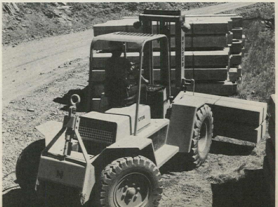
Sideloader can maneuver long loads like lumber down a narrow road or factory aisle. Jacks stabilize truck while mast extends sideways with load. Allis-Chalmers. CIRCLE READER SERVICE 275
