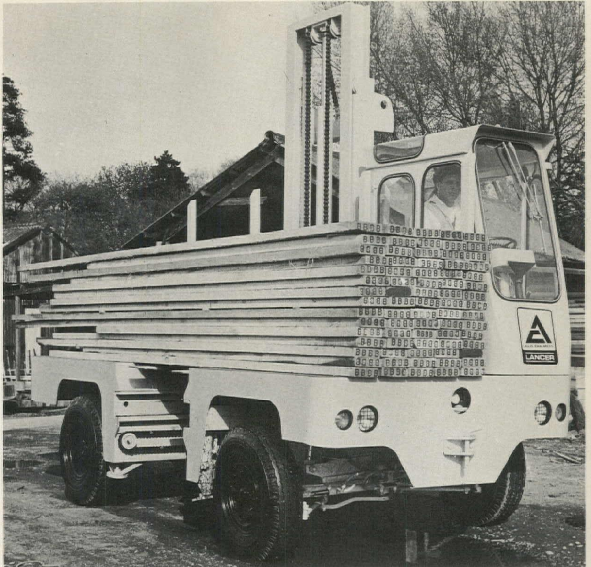
Sideloader can maneuver long loads like lumber down a narrow road or factory aisle. Jacks stabilize truck while mast extends sideways with load. Allis-Chalmers. CIRCLE READER SERVICE 275
