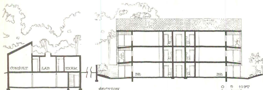
Sections show one-story medical building (left), and 2½-story apartments with balconies or sunken terraces.
