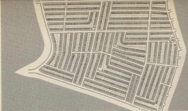
Land plan for Village Greens site was originally a conventional Staten Island grid (above). As laid out by architect Norman Jaffe, new plan (right) arranges 2,025 townhouse units in nine clustered villages, with plenty of open green area woven among them. Roads are excluded from greenbelt, and serpentine walks connect one village with another. Plan shows future sites of shopping center, schools, recreational facilities.
