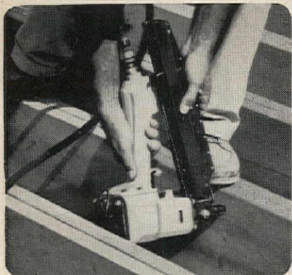
The Nailer drives 6d common to 16d sinker nails 5 times faster than a hammer.
