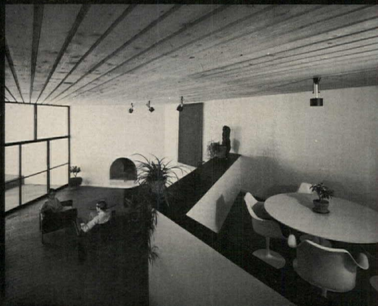
Raised dining area looks over living area and out through fully glassed end walls. Fireplace wall angles in to block western sun and wind.
