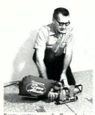
Seam cutter speeds floor laying, reduces fatigue, yet produces consistently even tight seams in sheet vinyl. Workman pushes tool across overlapped (no-pattern) flooring at 12' to 16' per min. A guide bar follows factory edge as 4" blade trims 1/2" from both edges. Armstrong, Lancaster, Pa. CIRCLE 224 ON READER SERVICE CARD
