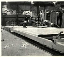
Roof panels are built continuously . . .
