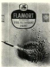
Fire retardant paint shields and insulates wood from flame, delays ignition. When exposed to fire, it bubbles and swells up to form a sponge-like insulating barrier, and it emits non-toxic fire-extinguishing gases that help to smother flames. After the fire is out and
