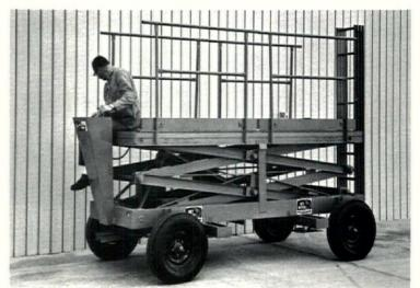
Mobile lift needs no tow truck, moves along with the job at up to 2 mph. Platform is 10'6" x 3'10", can be raised to a working height
