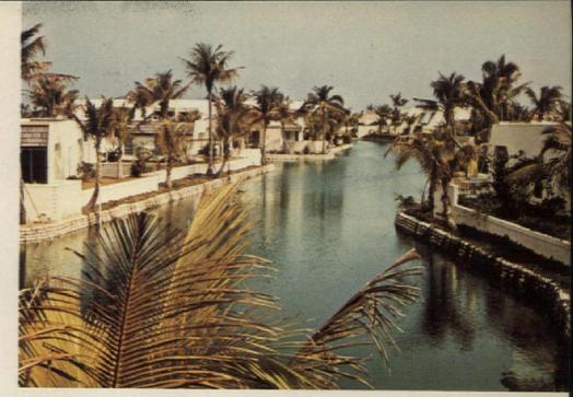
Narrow waterway (above right) gives the effect of a long canal, brings a feeling of unlimited space to the project. Rip-rap at edge of water is made of bagged concrete dropped in place and spiked down with reinforcing bars. Entrance and parking courts (right) are sited between each two rows of houses.
