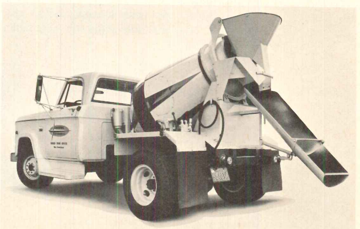
Small capacity mixer , only 78" wide and 84" high overall, has all the features of standard mixers. All hydraulic mixer, mounted on a one-ton cab and chassis truck, has a 6' discharge chute. Universal Fluid Dynamics, San Francisco. Circle 210 on Reader Service card
