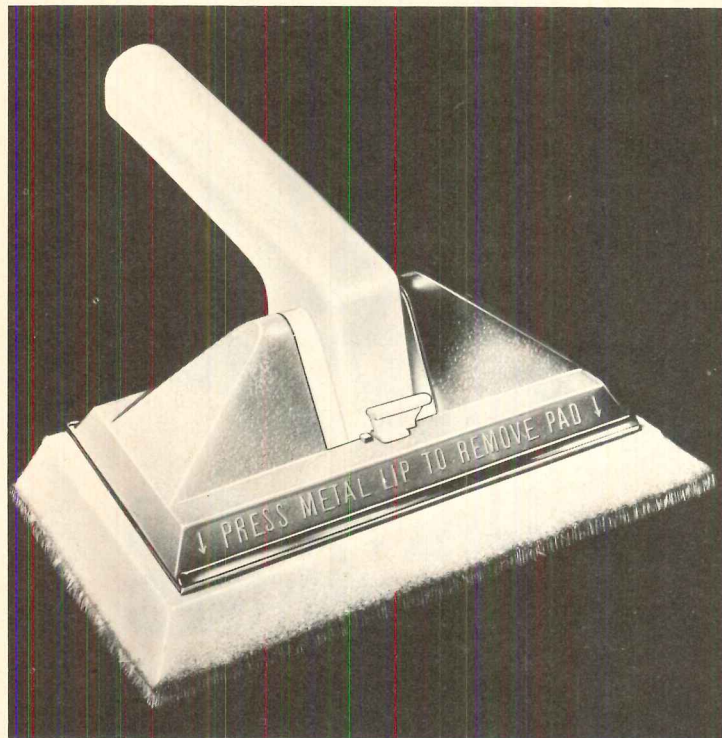
Paint applicator , primarily for outdoor work, gives a brush-like finish with the ease and speed of a roller. The 7"x4" flat nylon fiber pad holds enough paint to cover a 336-sq.-in. area, is replaceable. EZ Painter, Milwaukee, Wis. Circle 211 on Reader Service card
