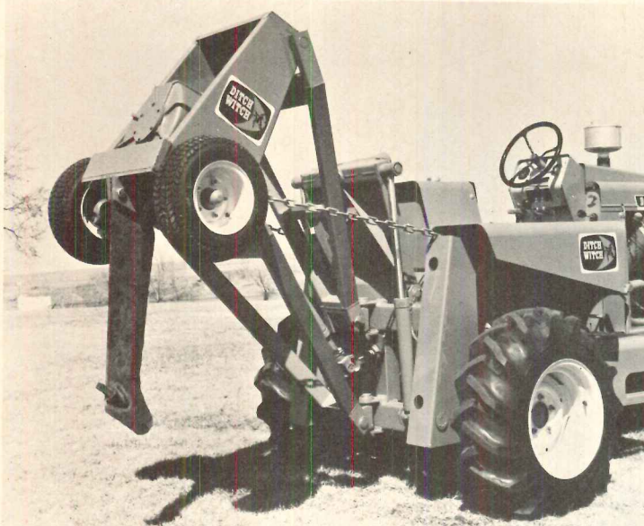
Vibratory plow attaches to trencher, installs cable underground without digging trench, threads cable into the ground. New isolated lift spring allows blade to vary depth while in operation. Charles Machine Works, Perry, Okla. Circle 204 on Reader Service card
