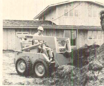
Compact loader is only 59" wide, 81½" long, can make a 360° turn in its own length. Four-wheel-drive unit with diesel or gas engine can lift up to 1,500 lbs. up to 9½' dump height, has 39 available attachments. J.I. Case, Racine, Wis. Circle 207 on Reader Service card
