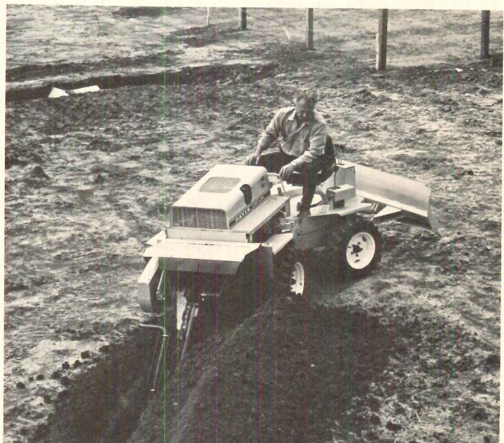
Articulated trencher , operated by one lever, digs a curved trench from 40" wide, 64" deep, to 12" wide, 30" deep, at up to 1,200 fph. Single lever controls speeds, forward and reverse, turns and braking. Davis, Wichita, Kans. Circle 209 on Reader Service card
