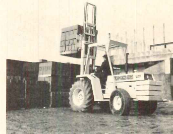
Fork lift with hydraulic transmission leaves operator's hands free for speedier, more precise control of lifting operation. Available from 4,000- to 5,000-lb. capacity, with wide range of attachments. International Harvester, Chicago. Circle 208 on Reader Service card
