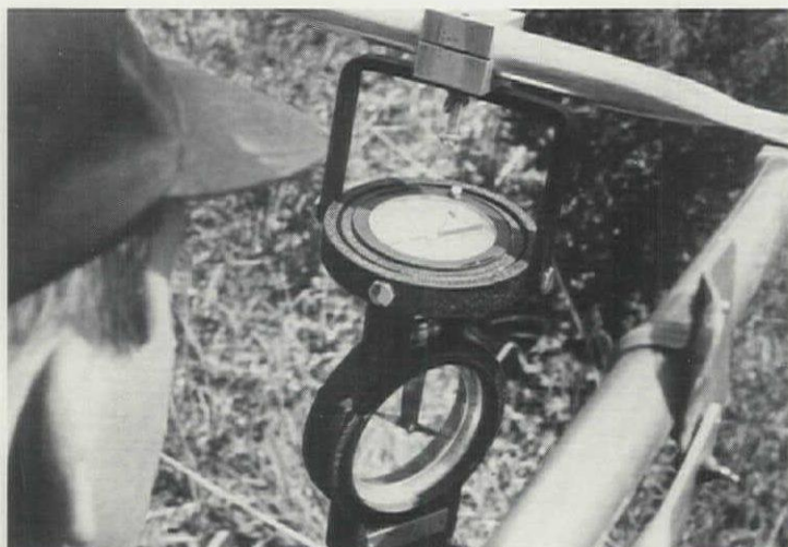
AQUATOMETER consists of two compasses: one, top, orients the instrument; the other reacts to changes in the earth's magnetic field underground.
