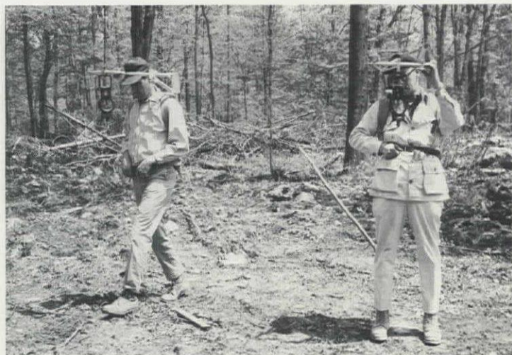
TWO-MAN TEAM uses Aquatometers to conduct water search. Readings are taken at 9' intervals; instruments are mounted on modified pack frames.
