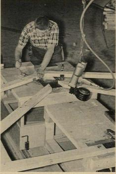
EXPANDABLE JIG for clinch-nailed trusses consists of roller-mounted tables on T-bar tracks.
