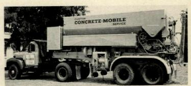
LARGE MODEL of 10-cu.-yd. capacity is mounted on a trailer and powered by auxiliary engine. Mixer operators are trained at manufacturer's factory.
