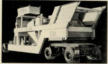
RUBBER-TIRE TRANSPORT carries compact concrete plant to the construction site. The equipment can be set up for full production within one day.
