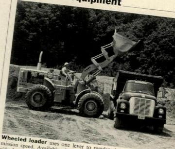
Wheeled loader uses one lever to regulate both direction and transmission speed. Available: four general-purpose buckets as well as rock, side-dump and multi-purpose buckets and a rear-mounted ripper-scarifier. Catepillar, Peoria, Ill. Circle 218 on Reader Service card
