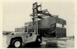
**MODIFIED FORKLIFT TRUCK** carries wrapped five-ton module from end of assembly line to specially designed flatbed trailer for delivery.
