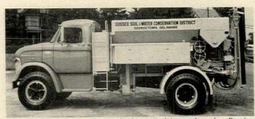
**SMALL MODEL** of 4-cu.-yd. capacity is powered by truck engine. Pouring rate is one cubic yard per two to four minutes, depending on type of mix.
