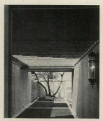
STREET SIDE has 6'-high wall on lot line to screen the entry and front patio. Mansard roof ties garage to house visually.
