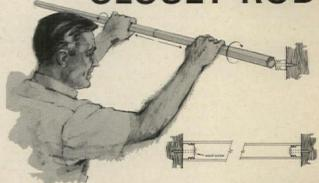
Seamless tubular zinc-plated steel rods slip over "end serts." Each "end sert" is a plastic anchor that attaches to wall with a single wood screw. A twist motion extends the telescoping rod flush with the wall surface.
