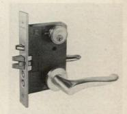
Mortise lock for lever handles features a three-piece latch-bolt with a full 3/4" throw. Nylon inserts in the guard bolt assure smooth operation. Eight designs come in brass, bronze, aluminum or stainless steel. Sargent, New Haven, Conn.
