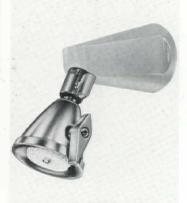
Non-scald showerhead made of triple chrome-plated brass with interior components of thermoplastic NORYL. Available with fixed or adjustable spray patterns, volume control, fixed-quantity flow restrictor. Symmons Engineering, Boston. Circle 251 on Reader Service card
