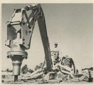
Hydraulic impactor-shown teamed with a tractor-backhoe-loader breaks pavement (above), tamps backfill, and drives posts or pilings. It can be installed quickly in place of the backhoe bucket. Ford Motor Co., Birmingham, Mich. Circle 217 on Reader Service card
