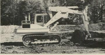
Hydraulic excavator with bucket capacity of 3/8 to 1/2 cu. yds. digs up to 16' deep (larger model digs to 191/2'). Wide range of optional equipment includes reversible buckets, clamshells and crane jibs. Massey-Ferguson, Akron, Ohio. Circle 215 on Reader Service card
