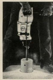
Rotary hammer with motor rpms and choice of light or heavy hammer blows is designed for continuous drilling in reinforced concrete without diamonds or water. Hammer drills 23" per min. on a ¾" hole. Black & Decker, Towson, Md. Circle 216 on Reader Service card
