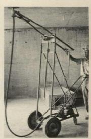
Gasoline-powered grinder with 9" abrasive disc grinds concrete ceilings from 7' to 11'3" high. Once height is set, operator pushing machine along can finish up to 500 sq. ft. per hour. Swivel top allows grinding close to walls. Stow, Binghamton, N.Y. Circle 218 on Reader Service card
