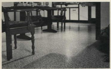
**Sheet-vinyl flooring**—in 12' as well as conventional 6' width—installs at any grade level without adhesive: Flooring is loose-laid and finished with quarter-round molding or vinyl cove base. Armstrong, Lancaster, Pa. Circle 222 on Reader Service card
