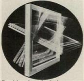
Double-glazed window comes horizontally or vertically pivoted, or side- or bottom-hinged. Of Swedish origin, window is made of wood faced with aluminum, copper or stainless steel; comes in a range of stock sizes. Wrand, Swarthmore, Pa.
