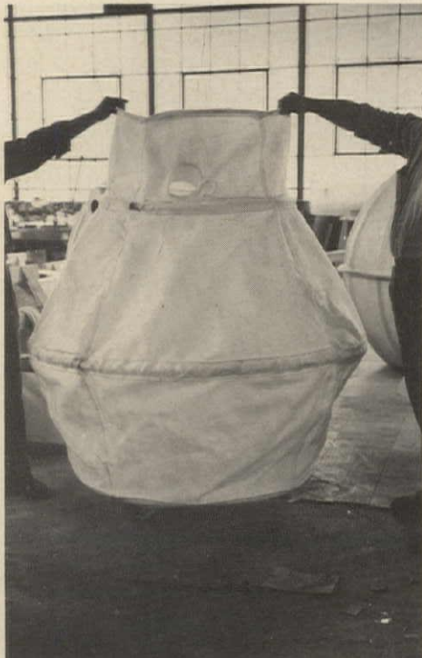
FILTER BAG of 50-micron plastic mesh passes only minute suspended solids for final outflow.
