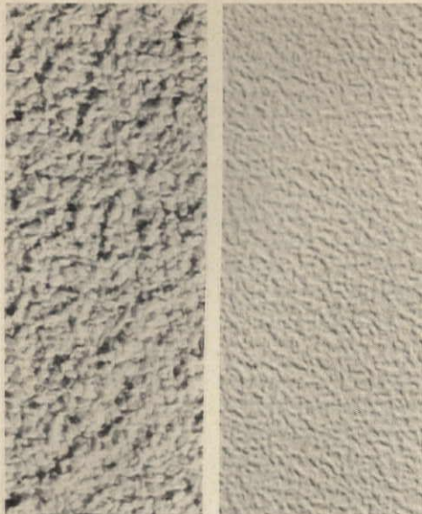
TEXTURED PLASTICS like Sanspray (left) and Weyerhaeuser Panel 15 add variety to siding.
