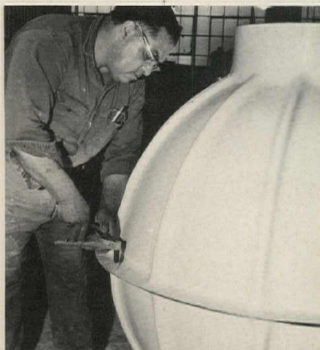
LIGHTWEIGHT SHELL of ribbed plastic is made in halves that nest for shipping and are fastened together with pop rivets. Besides the 600-gallon-per-day spherical size for individual houses, Cromar makes a 1,500-gallon-per-day cylindrical unit for gas stations and small restaurants ( shown in testing arrangement above ).
