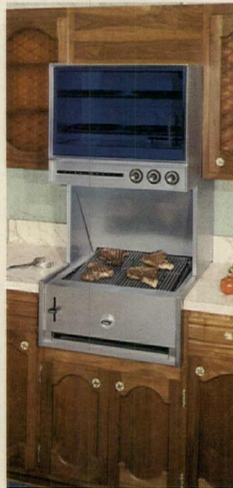
Set-on charcoal broiler combines concealed vent hood and eye-level warming oven in a single unit with one gas connection and standard duct. The two-piece, cast-iron grill fits into a dishwasher. Dyna Broil, Los Angeles. Circle 287 on Reader Service card
