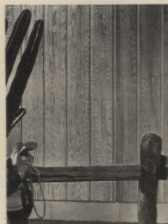
Textured siding made of abraded western Hemlock is straight-grained and incorporates 12" o.c. grooves 1½" wide by ¼" deep. It is available in 4'x8' to 4'x12' panels and is waterproofed on both surfaces. U.S. Plywood, New York City.
