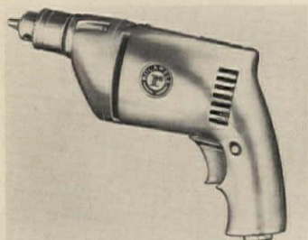
Variable-speed drill is trigger-controlled from zero rpm, thus eliminating center punching. Comes in 1/4" ($45) and 3/8" ($53) capacities. Both have 3-amp motors and ball and needle bearing construction. Rockwell, Pittsburgh. Circle 232 on Reader Service card
