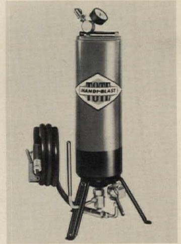
Portable sandblaster weighs 52 lbs filled, operates from 15 to 25 minutes with sand of 20 to 100 mesh size. Unit has steel pressure tank tested for 300 psi, and includes pressure gauge and relief valve. Lists at $155. Tote Systems, Beatrice, Neb. Circle 235 on Reader Service card
