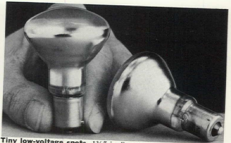
Tiny low-voltage spots , 1 3/4" in diameter, 2 5/8" long, are 15- and 25-watt, 12-volt reflector lamps. They fit some existing low-voltage equipment with single-contact bayonet base sockets. Design life: 2,000 hours. GE, Cleveland, Ohio. Circle 262 on Reader Service card
