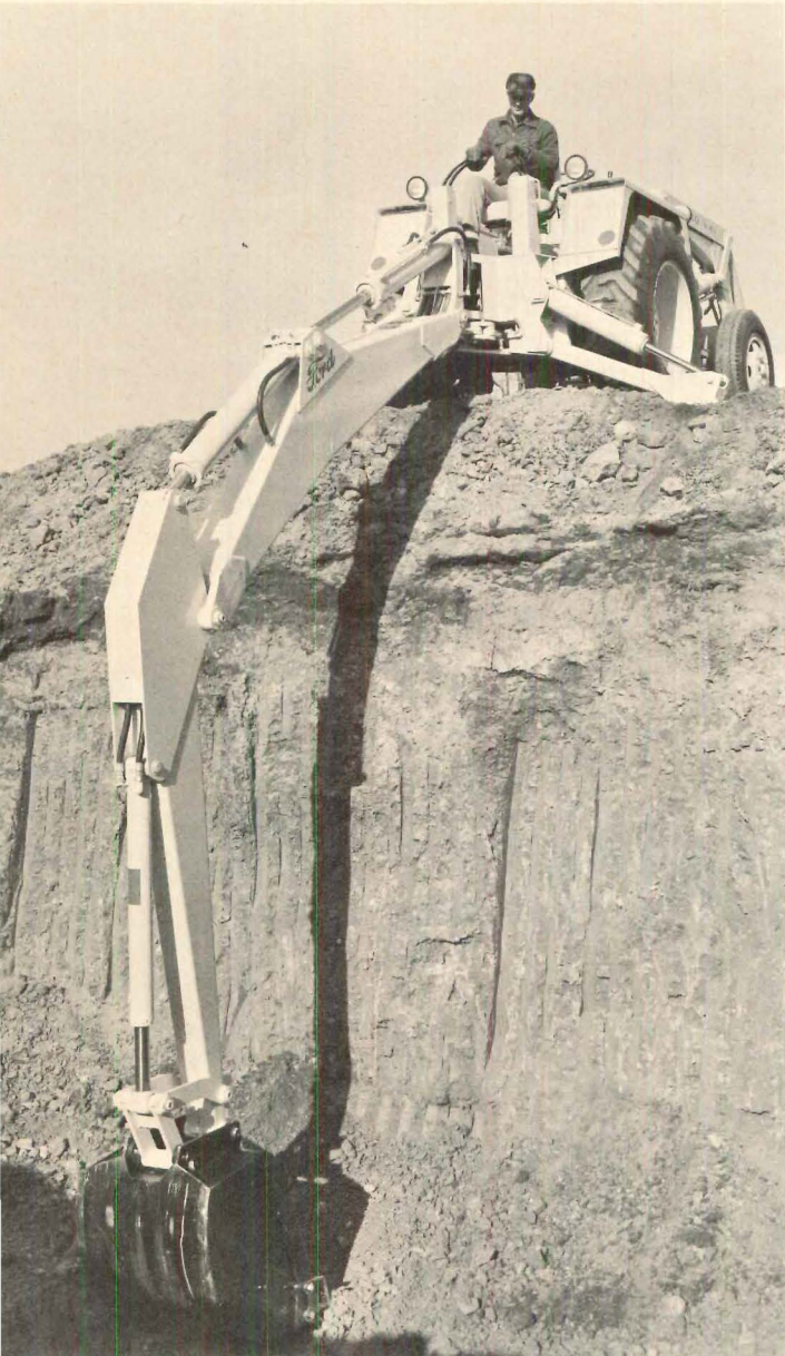
Backhoe-loader digs to depth of 17½'—or 2' more than maker's previous industrial units. Model No. 5500 is designed to meet growing demand for deeper digging. Heavier frame weighs 1¼ tons. Ford, Birmingham, Mich. Circle 234 on Reader Service card
