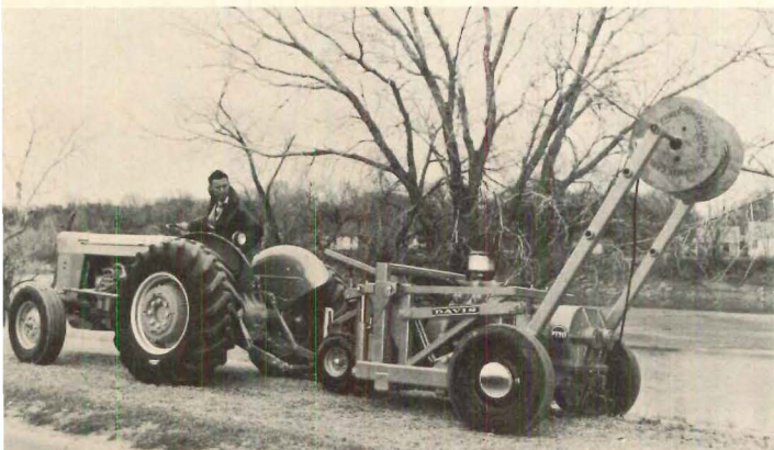
Knife-action cable-layer buries up to 1½" cable directly from reel without damage from knife vibration. Claimed speed for self-powered unit in optimum soil is 50' per min. at 30" depth. Davis Mfg., Wichita. Circle 232 on Reader Service card
