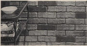
FIBERGLASS PANELS—48" wide and 10" high—are applied with just four nails. Patented, self-leveling and interlocking flange hides nail heads.
