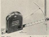
**Multi-purpose ruler** contains hinged point that converts ruler into a compass. An accurate circle can be drawn up to 12' in diameter by placing pencil point in hole at tape tip. Tape can be locked at any length. Custanite, Brooklyn. *Circle 266 on Reader Service card*
