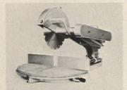
**Portable radial saw,** for wood, brick, stone, and aluminum, breaks down into two sections and fits in a car trunk. Saw cuts material up to 4" thick and 13" wide on 90° cuts and 9" wide on 45° mitre cuts. Port-A-Craft, Wetoma, Fort Worth. *Circle 265 on Reader Service card*
