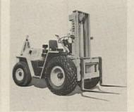
**Towable fork-lift truck,** with lifting heights to 16', incorporates a 109 h.p. engine, 13" clutch, and heavy-duty drive axles. The 14:00x20 drive tires provide broad surface contact for rough terrain. Capacity: 6,000 lbs. Champ, El Monte, Calif. *Circle 282 on Reader Service card*
