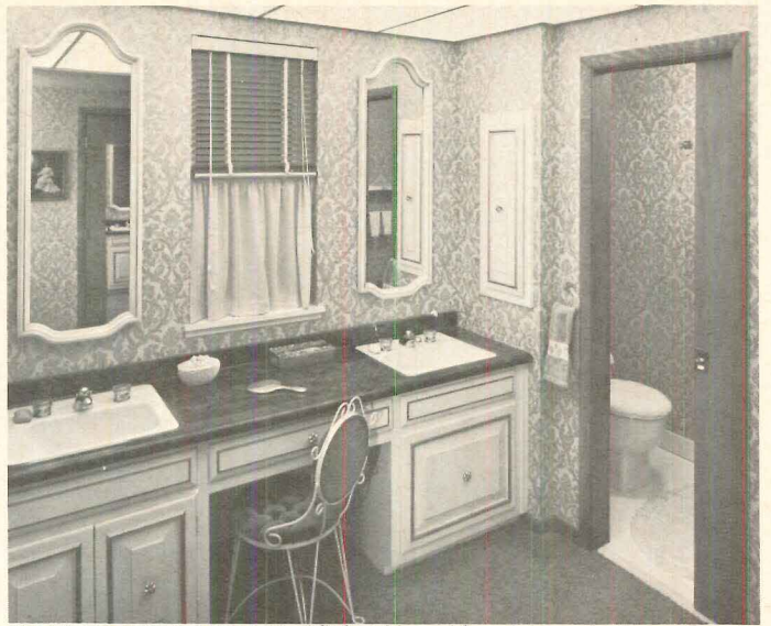
WALL-TO-WALL VANITY (6) has his-and-her sinks and mirrors. Luminous ceiling and window provide light. Pocket door at right saves space.
