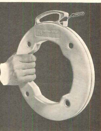
Fish-tape reel for pulling wire through conduit has molded-plastic housing and winder. Result: It is shockproof and half the weight of a steel reel. Tape sizes include 1/8"x100', 1/8"x200', and 1/4"x100'. Holub Industries, Plymouth, Ill. Circle 230 on Reader Service card
