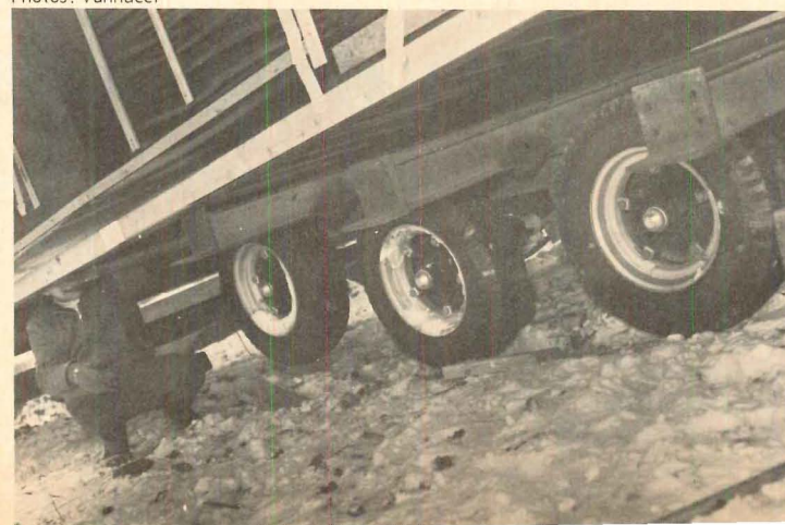
4. RUNNING GEAR is unbolted as section is jacked clear. Manufacturer retrieves gear later.
