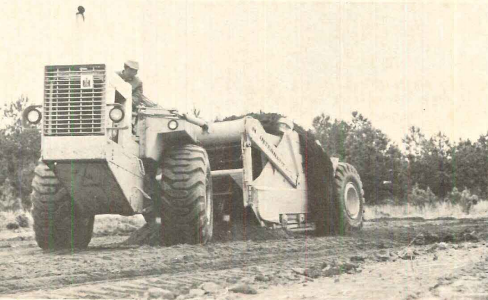
Leveling scraper. can travel at speeds up to 23.8 m.p.h. and make U-turn in 26'1". It permits a change of speed and speed range without declutching. Heaped-bowl capacity: 9 cu. yds. (10.8 tons). International Harvester, Chicago. Circle 220 on Reader Service card
