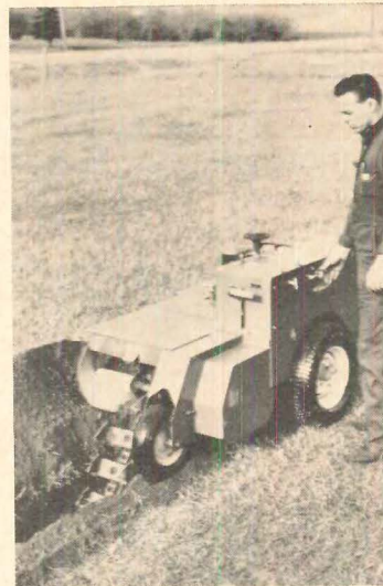
Self-propelled trencher digs 12"-wide trench 3' deep, or 4"-wide trench 6' deep at speeds up to 20' per minute. The 18 h.p. machine is 64" long, 25" wide. Digging chain is 20,000-lb test; teeth are replaceable. Wind-King, Merrill, Iowa. Circle 251 on Reader Service card
