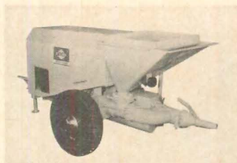
Concrete pump can be used for both conveying material and wet-gunning. Average pumping rate is 20 cu. yds. per hour over distances of 400' to 500'. Manufacturer's line also includes a pump-and-spray machine for plaster. Mayco, Los Angeles. Circle 256 on Reader Service card
