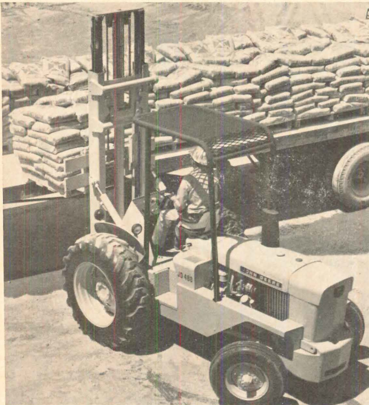
Heavy-duty forklift comes with choice of 14' or 21' mast. Full-height load capacity is 2,500 lbs. with taller mast, 5,000 lbs. with shorter mast. Engine size is 59 h.p., with eight speeds forward, eight reverse. John Deere, Moline, Ill. Circle 250 on Reader Service card.
