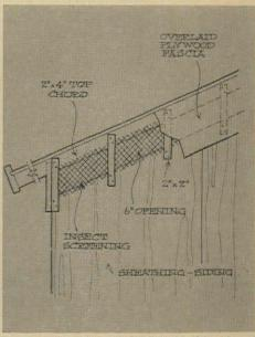
insect screen and concealed by wide frieze board on 2x2 spacers. Frieze is cut from overlaid plywood which is prestained in on-site shop.
