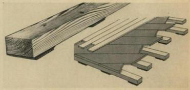
**Cushion-soled sleepers** are screeds which, when placed on 12" centers above a moisture barrier on a concrete slab, serve as nailers for subfloor and finish floor. The sleepers come in 3', 4', 5' and 6' lengths. Potlatch, San Francisco. (Circle 215 on Reader Service card)
