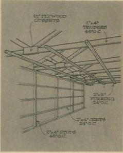
under floor joists would have required 2x8 header. Cost difference between new and conventional wall-framing systems is not significant.
