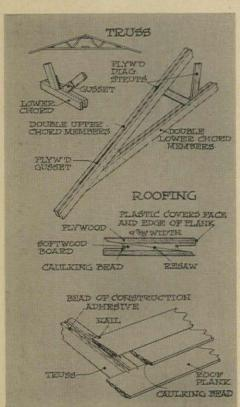
ROOF SYSTEM is framed by sandwich trusses, finished by laminated boards with lapped joints.
