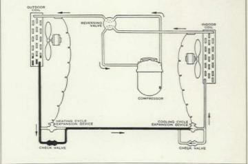
CONVENTIONAL COOLING CYCLE is regulated with expansion valve.
