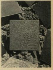
Cement bonded tile comes in square and hexagonal shapes 53/4" x 53/4" with a recommended 1/4" joint. Franciscan Promenade tiles are available in a wide range of colors with matching grout. International Pipe & Ceramic Corp., Los Angeles.
