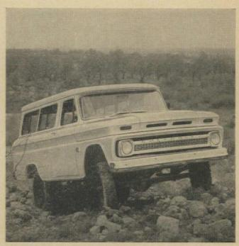
Suburban Carryall 4x4's offer you a choice of panel or station-wagon-type rear doors; they're unbeatable as back-country crew and equipment carriers. Wheelbase is 115". Also available are a 7½-foot panel model plus ½-ton and ¾-ton chassis-cab models.
