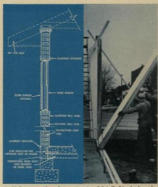
(Left) Cross section shows structural detail of typical modular panel unit positioned on pre-installed footings and floor. (Right) Wall panels are aligned and fitted into pre-caulked and drilled metal channel, secured with self-tapping screws.
