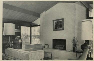
FAMILY ROOM INTERIOR has a cathedral ceiling with wood planks supported by transverse beams. All interior walls are finished in wood.
