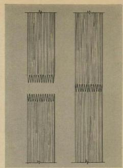
**END-GLUED FRAMING**, used in truss chords, is a product of impression finger-jointing machinery operated by seven Western lumber firms.
