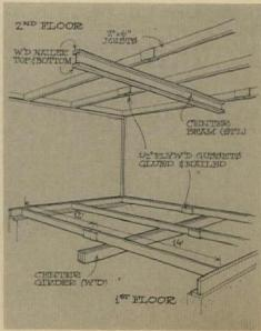
combined with %" t&g glue-nailed subfloor. Splice joints, produced in NAHB's lab, were safely loaded with 1,000 lbs. Floor holds 180 lbs. per sq. ft.
