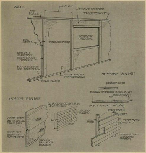
WALL SYSTEM combines three glue-laminates: stud-fiberboard, siding-sheathing, drywall-stiffeners.
