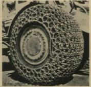
Protective chains for wheel tractors reduce tire wear in rocky soil by shielding tread and side walls from objects over 3" in diameter. Chains may be turned over for longer wear. Tire sizes: 29.5x29, 33.25x35, 20.5x25, 17.5x25. Caterpillar, Peoria, Ill.
