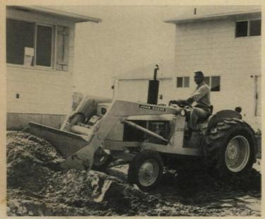
Low-profile wheel loader offers choice of three bucket sizes, diesel or gas three-cylinder engine, eight forward and four reverse speeds to 16.2 mph. Breakout force: 3,000 lbs. Lift capacity: 2,000 lbs. to 9'9". John Deere, Moline, Ill. (Circle 224 on Reader Service card)
