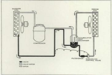
NEW COOLING CYCLE for heat pumps introduces heat exchanger control.
