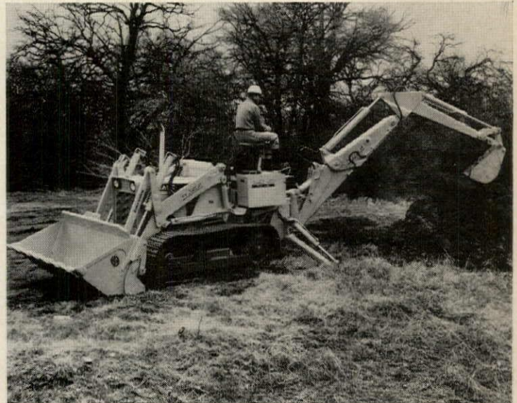
Light tractor-crawler has a torque converter, one-hand power shift and power shuttle, turning and steering. Attachments include a 4,500-lb. capacity loader, a 14' backhoe, ripper, guards, winches and others. J. I. Case, Racine, Wis. (Circle 218 on Reader Service card)
