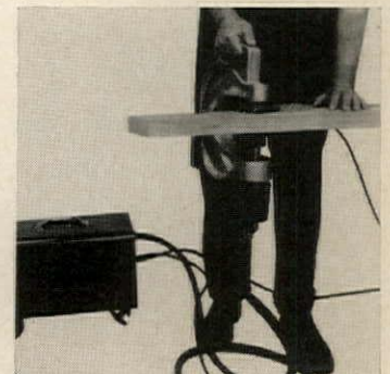
Truss press clips on both sides simultaneously so truss needn't be turned over. Operating on 110 volt current, the unit can be used on or off the site. Aluminum jaw has an 8" throat allowing usage on most truss types. Panel-Clip, Farmington, Mich. (Circle 221 on Reader Service card)
