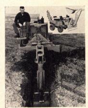
**Backhoe** attachment double action in the backhoe arm allowing the bucket to be folded back over the trencher. The hydraulic attachment is available in 12", 18" and 24" sizes. Backhoe is detachable. The Charles Machine Works, Perry, Okla.
