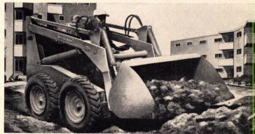
**Small loader** has a hydraulic front-end drive with separate motors on right and left wheels to permit accurate turning. The 30 hp engine is air cooled. Unit can accommodate 1,500 lbs. Erickson Power Lift, Minneapolis. (Circle 231 on Reader Service card)
