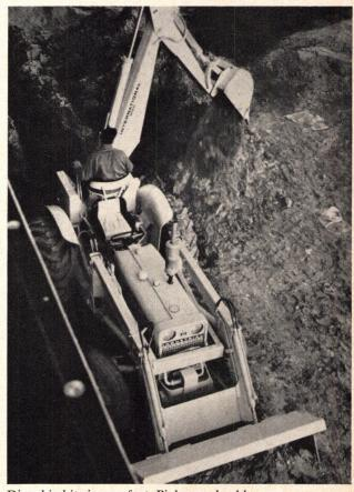
Dig a big bite in comfort. Pick your backhoe: 16' reach with 13' digging depth, or 17' reach with 14' depth. Only split console on the market. Makes plenty of room for legs and feet. No hot housing to straddle.
