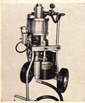
Airless paint sprayer can deliver up to three gals. per minute to five guns. Unit has a siphontype pump on a tubular dolly for mobility. A five gal. container carried on the dolly or a 55 gal. drum can supply paint. Spee-Flo, Houston.
