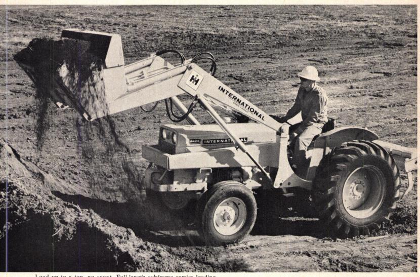
Load up to a ton-no sweat. Full-length subframe carries loading shocks direct to rear axle carriers. Protects engine and power train. Visibility? Unbeatable. Towers are  $6\frac{1}{2}$ " lower than earlier models.
