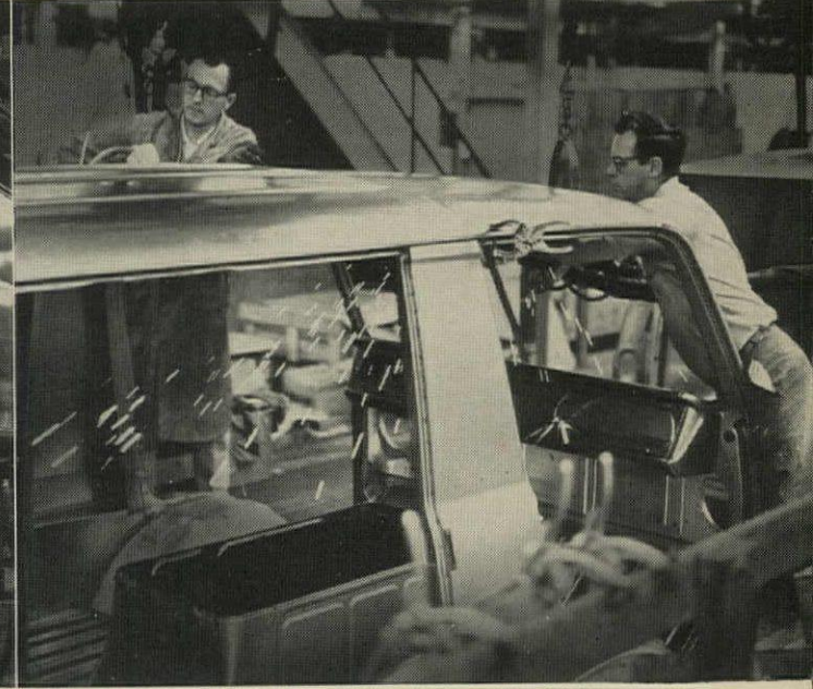
followed by front end panels, many galvanized ... and a ribbed roof panel caps the structure.
