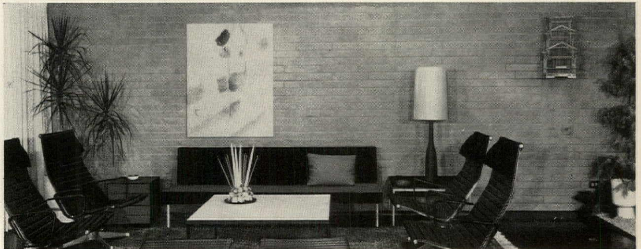
Attractive concrete split block of interior walls provides intriguing, rough-textured background for furnishings. Truncated pyramid ceilings have central skylights.
