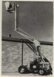
**High-lift loader** is one of ten models with reach heights up to 40' and capacities of 2,500 to 6,000 lbs. Accessories include concrete hoppers, hod buggies, buckets and workman's platforms. Lull Engineering, St. Paul, Minn.
