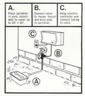
\$100 Moist O'Matic system like this installs in two man hours. Sprinkles 50' x 50' area.
