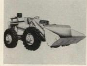
Wheel loader has two-cu.-yd. capacity with a 10,000 tipping load. Model W8B has a 45° bucket rollback at ground level and a 53" reach at 7'. Steering shifting, shuttling and braking are all power controlled. J. I. Case, Racine, Wis.
