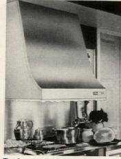
**Barbecue hood** has removable scalloped trim, aluminum filter, two-speed exhaust fan (600-800 cfm) and fluorescent lamp. Char-Grill hood, 30" high, 30" wide and 24" deep, can be back or top-vented through wall or ceiling. Majestic, Huntington, Ind. *Circle 15 on Reader Service card*
