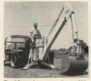
**Backhoe** is mounted on  $1\frac{1}{2}$ ton truck for speed and mobility. Model 180 Truck Hoe uses hydraulics to move itself off and on the truck bed. It has a  $16\frac{1}{2}$ ' reach, can dig to a  $13\frac{1}{2}$ ' depth. Seven different buckets are offered. Henry Mfg., Topeka, Kans. *Circle 89 on Reader Service card*
