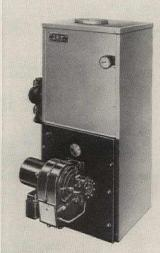
Low-cost boiler of cast iron has a built-in tankless water heater. Oil-fired APT unit provides from 95,000 to 165,000 btu, is packaged with prewired controls. It can be installed in a 291/2"x 311/2" space. American-Standard, New York City. Circle 118 on Reader Service card
