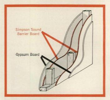
intermediate studs. All vertical joints are finished in the normal way. This system gave an STC rating of 45 and when tested according to ASTM E119 achieved a 70-minute load-bearing fire rating plus the hose stream, double-load test. For full information on this remarkable new product, see your Simpson Building Products supplier or write to the address below.
