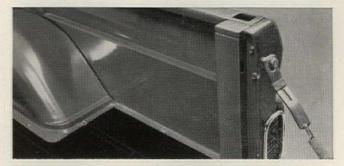
**DOUBLE-STRONG BODY AND CAB** Double-walled cowl arch, double-paneled roof and double-braced floor panels make Chevy pickups quieter, stronger and longer lasting. Independent front walls on Stepside and Fleetside bodies isolate cab and driver from the battering of shifting loads. Double-wall construction of lower body panels in Fleetside models keeps dents on the inside, not the outside.
