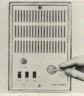
**Home intercom** is transistorized for compactness, will handle up to 16 stations and can be surface or flush mounted. It requires a wall opening only 2" deep by  $6\frac{1}{2}$ " high by  $4\frac{1}{8}$ " wide. Front is stainless steel. Talk-A-Phone, Chicago.
