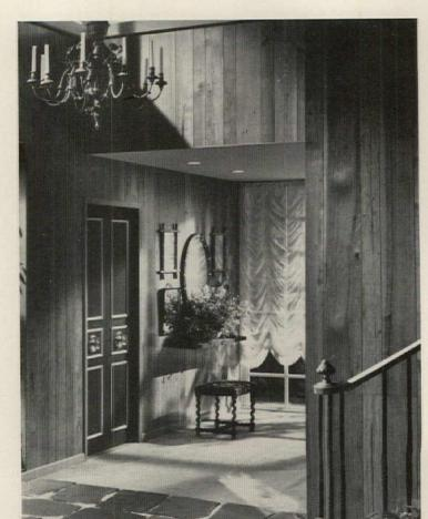
**Hickory paneling** is a new addition to this manufacturer's Craftsman line of medium-priced, prefinished plywood paneling. It is offered in 4'x7' and 4'x8' sheets with a V-groove pattern. U.S. Plywood, New York City. (*Circle I on Reader Service card*)
