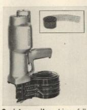
**Canister nailer** drives fullhead, standard 6d or 8d common, box or sinker nails. Nails are packaged in coils of up to 300. Model N2 Common Nailer has touch-trip, semi-automatic or fully automatic control. Bostitch Inc., E. Greenwich, R.I.
