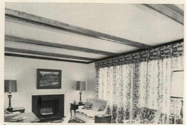
Large modular panels, available in 4' widths and in lengths up to 16', are made of Fiberglas acoustical insulation faced with white embossed vinyl film. Panels absorb 60% of noise striking them. Owens-Corning Fiberglas, Toledo, Ohio. (Circle 30 on Reader Service card)
