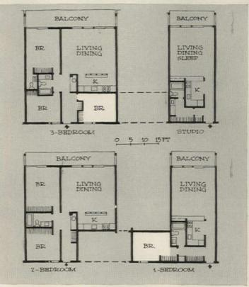
**ONE-LEVEL PLANS** with interlock design would permit easy altering of apartments (*broken lines*).
