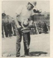
Utility breaker can be used to remove old concrete floors or stone or to loosen compacted soil, clay or gravel. In addition, model UB-25 can be used for tamping, pipe laying and post setting. Wacker Corp., Hartford, Wis.
