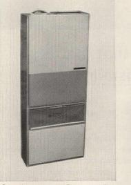
Apartment unit combines heating and cooling in a 26"x 12"x72" cabinet. Combustion gas and condenser air are exhausted through the wall. Heating capacity is 40,000 to 60,000 btu, cooling capacity is 11/2 or 2 tons. C. A. Olsen Mfg., Elyria, Ohio. Circle 117 on Reader Service card
