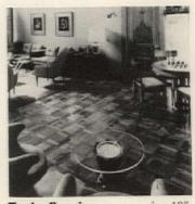
**Teak flooring** comes in 18" squares with a paper face (to be removed after installation in mastic). Six patterns are offered at list prices ranging from \$1.16 to \$2.58 per sq. ft. Nosings, saddles and moldings are available. Bangkok Inds., Philadelphia. *Circle 39 on Reader Service card*
