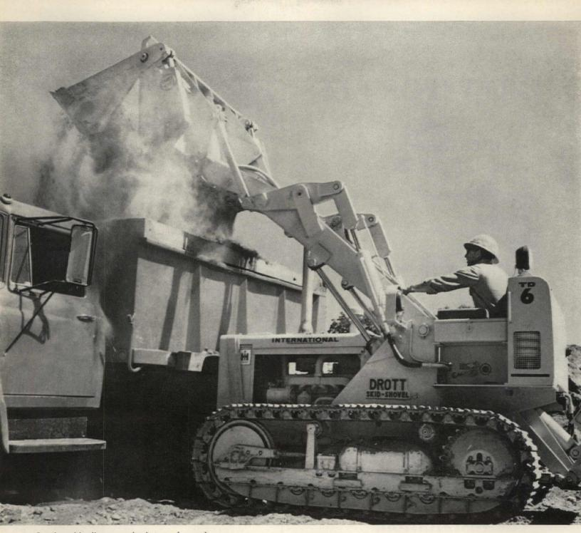
Loader with all-purpose bucket can be used as a dozer, a scraper, a loader or a clamshell.
