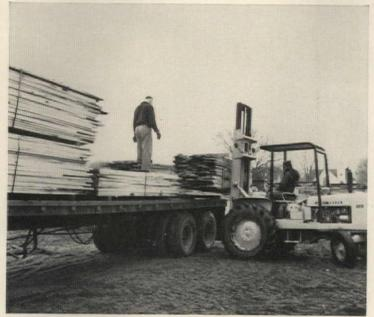
**High-lift forklift** comes with a 21' mast that has 2,500 lb. capacity at full height, 5,000 lb. capacity at 14' height. Also available: interchangeable hydraulic bucket, mortar hopper, blade and swing boom. John Deere, Moline, III. (Circle 74 on Reader Service card)
