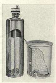
**Commercial water softener** can handle flow rates up to 40 gals. per minute without excessive loss in water pressure. It has 11/2" ports and a 450-lb. salt storage tank. Capacity is up to 90,000 grains per regeneration. Culligan Inc., Northbrook, Ill. Circle 125 on Reader Service card
