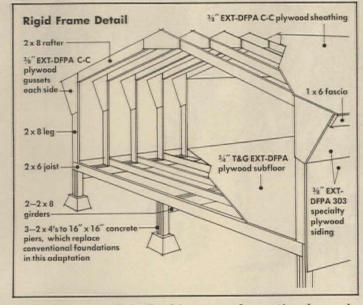
Ralph Grinnell built this unusual vacation home in Wollochet Bay, Wash., at a cost of less than \$1,000 for materials. It took just six days, from footings to painting. He used the rigid frame system. It's based on one simple component that combines functions of studs and trusses (see diagram above). Rough-sawn plywood sidewalls lock frames into a rigid, non-racking structure.
