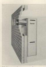
**Chimneyless gas furnace** has concentric through-wall flue to take in fresh air and exhaust combustion air. Saf-T-Sealed unit has 55,000 btu heating capacity, can also be fitted with a two-ton cooling system. Peerless Div., Louisville, Ky.
