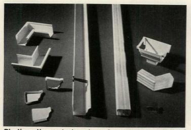
**Plastic gutters** and other rain-carrying components are made of white rigid vinyl, hung with metal hangers and downspout brackets. Gutter sections and end caps are solvent-welded together and snapped into hangers. Monsanto, St. Louis. (*Circle 43 on Reader Service card*)
