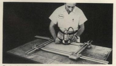
**Router template** puts complete ornamental design on cabinet doors in less than 30 seconds. Ten different guides are offered and each can be used on doors as small as  $3\frac{1}{2}$ " x  $3\frac{1}{2}$ " or as large as 24" x 36". Wing Products Co., Scottsdale, Ariz. (Circle 80 on Reader Service card)
