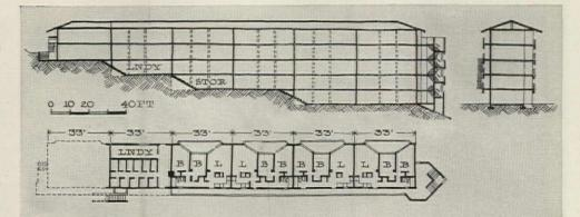
SECTION AND PLAN show how long, narrrow buildings were sited at right angles to slope.
