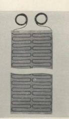
**Electric heat mat** is designed to be embedded in concrete floors, can be installed in one pour. Mats 16" wide by 10' long can be laid in corners or curves. They provide 20 watts per sq. ft., use 120, 208 or 240 volts. Easy Heat, Lakeville, Ind.
