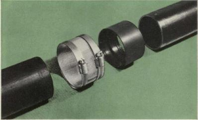
The durable **NO-HUB** joint for pipe and fittings. Utilizes a Neoprene sleeve gasket over joined ends, and a protective stainless steel shield held firmly in place by stainless steel bands permanently fastened by worm drive clamps. Below ground or above floor, this joint does not corrode or deteriorate; remains gastight and watertight. It's strong; not affected by shock or vibration.
