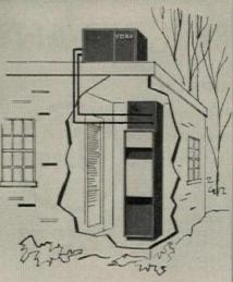
Ranch home application. Exhaust section is outside, on slab. Horizontal furnace and coil are located in attic space.
