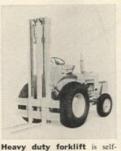
propelled, comes with lift heights ranging from 10<sup>1</sup>/<sub>2</sub>' to 21<sup>1</sup>/<sub>2</sub>'. High flotation tires and improved underaxle and undermast clearance help machine withstand extreme loads. International Harvester, Chicago.
