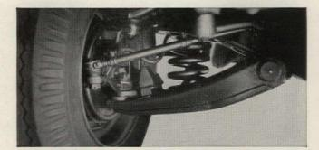
SMOOTHEST OF TRUCK RIDES-NOW WORK-PROVED! Chevrolet pickups feature independent coil-spring front ends teamed with two-stage coil or leaf-spring rear suspensions. Both systems provide top payload capacity with special ride smoothness. And both are work-proved for maximum reliability, top Workpower.
