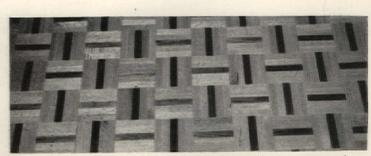
**Hardwood flooring** comes in 19" x 19" paper-faced squares made up of sixteen 4<sup>3</sup>/<sub>4</sub>" squares with four light and one dark hardwood slat. Panels can be mastic-installed over concrete or wood. Harris Mfg. Johnson City, Tenn. (*Circle 33 on Reader Service card*)
