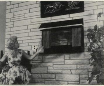
**Barbecue-fireplace** is prefabricated of stainless and aluminized steel. It includes a chimney, motorized spit and log grate. Designed for thruthe-wall installation, it requires zero clearance. Waste High Fireplaces, Kansas City, Mo. (*Circle 127 on Reader Service card*)
