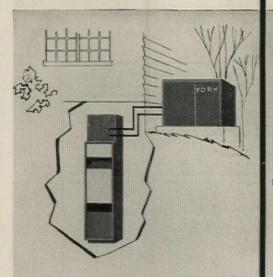
Roof location. In this gardentype installation, outside section is on roof. Furnace and coil are in alcove.
