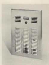
Wall air purifier removes odors by drawing air through a charcoal filter. It can be operated intermittently or continually. Models have 150 or 300 CFM capacity, operate on 115 volts and can be set in a 4" wall. Barnebey-Cheney, Columbus, Ohio.
