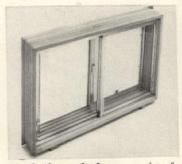
**Insulating windows** consist of two aluminum-framed sliding units set in a wood frame to eliminate condensation. Windows are weather stripped with vinyl on the outside and wool pile inside and have aluminum screens. Ida Products, Detroit. *Circle 53 on Reader Service card*
