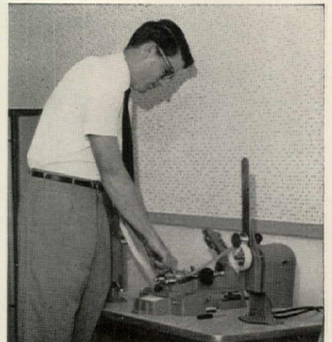
Tape is spliced as it leaves accounting machine.
