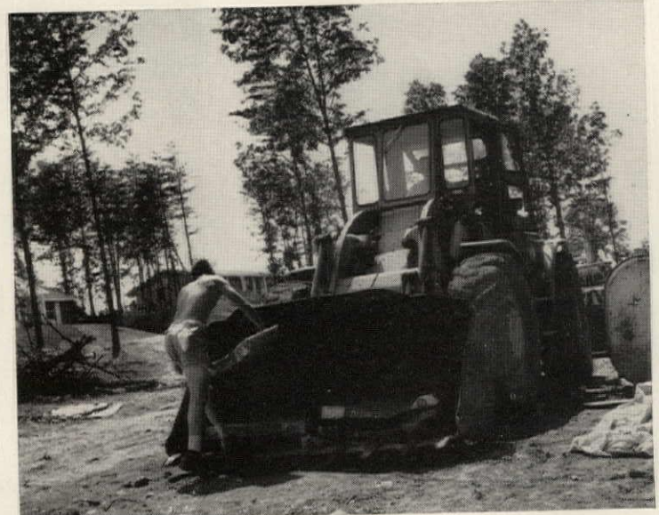
BIG LOADER also doubles as materials-handling machine. Here it picks up the shingles for an entire house, will carry them to the job over ground that is too rough and muddy for the supplier's truck. Brosius estimates that his earth-moving machines save an average of $100 a house this way.
