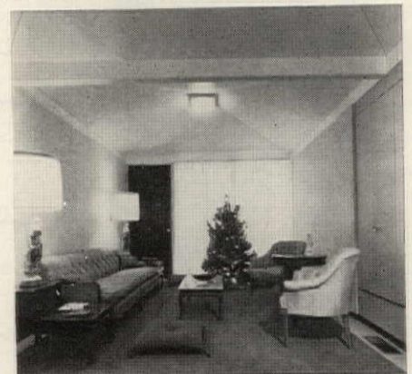
Spacious feeling of interiors stems from height of roof pyramids (10' at peaks). Floor area was also gained by cantilevering closets, right, beyond exterior walls.
