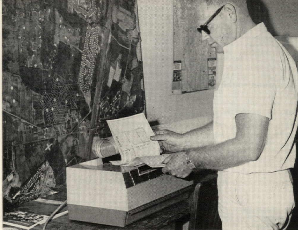
Floor plans are reproduced on white paper which picks up every detail.
