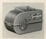
High-output humidifier has a capacity of 16.6 gallons of water a day. V-11 vapor wheel has a slowly revolving polyurethane-foam wheel as an evaporator surface, costs less to run than a 60-watt light bulb. Lau Blower Co., Dayton, Ohio.
