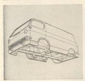
Tough unitized structure is formed of heavy-gauge steel to give a tight, rattlefree unit that will withstand the rigors of the toughest hauling schedules. Critical underbody areas are specially treated to ensure long-lasting corrosion resistance.
