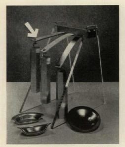
**STRENGTH TEST** shows stiffness of new laminate (arrow) vs. reinforced plastic and steel.
