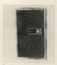
Fan-forced heater for in-wall installation is rated at 1,500 watts for either 120- or 240-volt operation. Separate rough-in box permits fast installation of heater with only four screws, Lists for \$34.95. Arvin Industries, Columbus, Ind.
