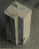
**Framing parts** are manufactured at mill. Stud-tee (*top*) is used at wall intersections. Corner-post (*bottom*) is used for either inside or outside corners. Priced slightly higher than raw lumber, both parts are 8' long. Potlatch, Warren, Ark.
