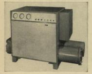
Water chillers for high-capacity cooling systems are packaged in units only 35" wide and 6' 8" long—small enough to go through a standard exterior door. Airtemp units are rated from 20 to 100 hp., operate with a single compressor. Chrysler, Dayton. For details, check No. 31 on p. 203
