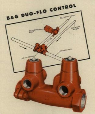
In primary-secondary systems equipped with Duo-Flo Controls, secondary zones are always controlled, even with high head pumps in the primary zone. Use of higher temperature drops permits sizable reduction in pump horsepower. Material saved includes 2 Flo-Control Valves, 2 shut-off valves, 2 or 3 tees and 6 nipples.
