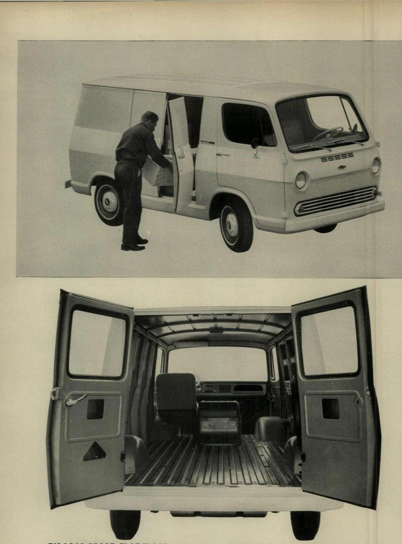
**BIG LOAD SPACE, FLAT FLOOR.** Cargo area is 7½ feet long—with an extra 4 feet of length along the right side of the engine. Interior height is 54½". You get 211 cubic feet of capacity in all. **EASY TO LOAD OR UNLOAD.** Those big rear and side doors are over 4 feet in both width and height to make it easy to load big bulky items. Rear windows and side doors are optional at extra cost.
