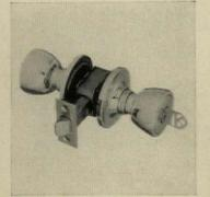
Heavy-duty lockset is made of steel and brass. Designed for custom houses, apartments and light commercial buildings, it meets federal specification 160. Half-inch latchbolt throw eliminates need for close door fit. Kwikset, Anaheim, Calif. For details, check No. 17 on p. 198
