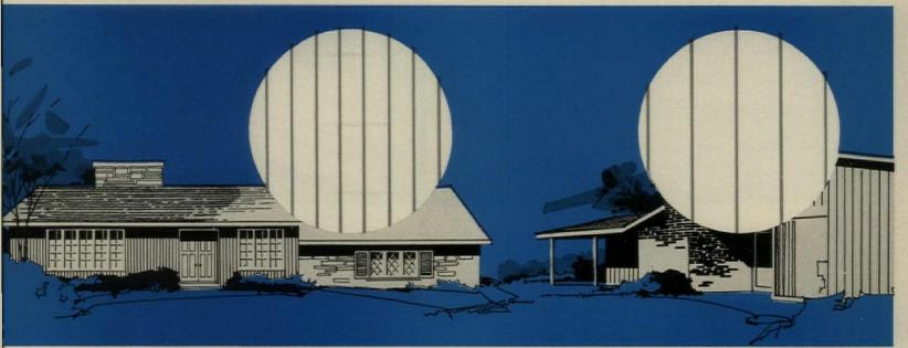
Shadowcast 4" U-Groove Siding-Vertical grooves spaced 4" o.c.; Shiplap joints on long edges of panels. Nominal %6" thick; 4' wide, lengths to 16'.
