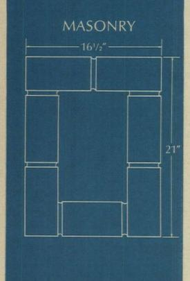
**BLUEPRINT COMPARISON TELLS THE STORY.** Competitive devices never get off the ground in the race to save builders space. Cross section comparisons show 7-K trims the bulk off a residential chimney. In a ten-foot installation, 7-K would consume only seven cubic feet of space compared to 12 cubic feet for ordinary factory-built chimneys and 36<sup>1</sup>/<sub>2</sub> cubic feet for masonry.
