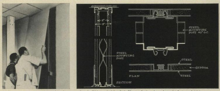
STEEL-AND-GYPSUM PANEL snaps into place on steel studs. Wiring and piping fit in 2" core. Section above shows detail at panel joints.
