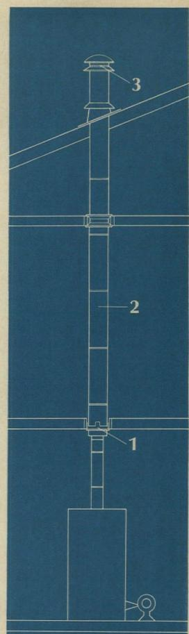
**INSTALLATION AS EASY AS 1...2...3.** (1) Support plate installs between joists and starter section provides first foot of 7-K Chimney. (2) 7-K Chimney pipe TWIST-LOCKS together, no rings, no cement, no screws. Guaranteed one-man installation. (3) A contemporary, enamel-finished top, scientifically designed to prevent roof staining. It's water tight and corrosion resistant.
