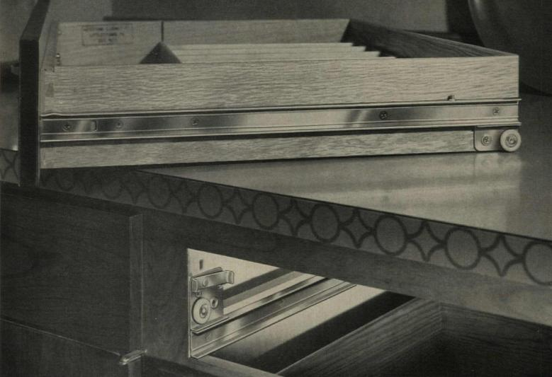
K-V 1300 Drawer Slide. For loads to 50 pounds. Only ½" clearance required each side. Nylon ball-bearing wheels give smooth, noiseless, lifetime operation. Economical, easy to install. Bright zinc-plated finish. Sizes from 12" to 28".
