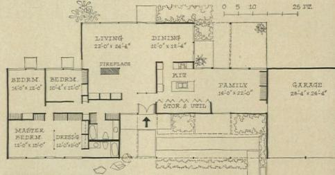
**FLOOR PLAN** shows wide degree of flexibility that is obtained from just two basic panel lengths—12' and 14'.
