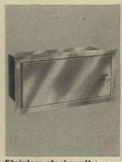
Stainless-steel vault to protect valuable papers from fire and theft is installed in place of one concrete block. 30-min. tests showed inside temperatures did not exceed 250F when temperature outside was 1,800F. Construction Products, New York City. For details, check No. 27 on p. 165
