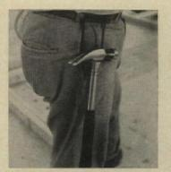
**Hammer holster** will end torn pockets and broken coverall loops. It can be hooked over a belt or looped on the ties of a nail apron. The holster is made of heavy wire coated with plastic to prevent rusting and scratching. Weyerhaeuser, Tacoma.
