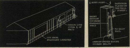
Drawing, left, shows layout (16" or 24" o.c.) of strips on sheathing. Fastening and butt system is shown at right.
