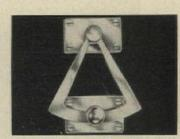
**Dutch-door quadrant** of solid heavy forged brass comes in dull and polished brass, dull and polished chrome, and dull bronze. A nylon washer provides tension and lubrication for firm holding and no rattle. Size: 4"x43/4". Baldwin Hardware, Reading, Pa. *For details, check No. 21 on p. 165*
