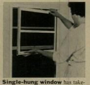
out vent for easy cleaning. Aluminum frame has white-bronze cam-type lock, vinyl glazing bead, flashed integral fin trim, screen retainer channel, step sill, and wool-pile weatherstripping. Miami Window Corp., Miami. For details, check No. 11 on p. 155
