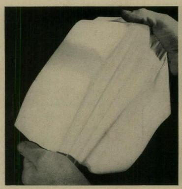
TEDLAR\* PVF film is a tough new filmfinish—not a liquid or a spray. TEDLAR is factory-bonded with special Du Pont adhesives to wood or metal, actually becoming part of the material it protects.
