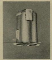
Ceiling-mounted heater draws fresh air from attic, heats it to room temperature, and injects it into the living area. Tempered Air Inlet extends 10" into the attic, has 7" fan and 1400-w. heater. Retail price: \$69.95. Arvin, Columbus, Ind.
