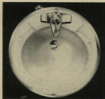
Vitreous-china bowl with integral soap dish, concealed-front overflow, and anti-splash rim is 18" in diameter. It comes with 4" centers for single-handle fitting (shown) or 8" centers for other fittings. White or six pastels. Kohler Co., Kohler, Wis. For details, check No. 13 on p. 206
