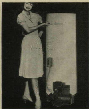
Oil-fired water heater has recovery rate of more than 60 gal. per hr. The M-40 has a glass-lined heavy-gauge steel tank, adjustable temperature control, and requires only a 4" flue opening. Ten-year guarantee. Glass-Lined Heater, Cleveland. For details, check No. 15 on p. 206
