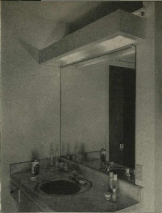
SUSPENDED LIGHTING PANEL bounces general lighting from ceiling while providing a good shaving light at the counter. Builder: Whitecliff Homes, Oakland, Calif. Designer: Edward Hageman.
