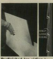
**Prefinished lap siding** has a Videne plastic surface and a hardboard base. A slanted lockstrip runs along the bottom edge of each course, fits into the beveled top edge of the course below. Color-lock is 12"x12"x7/16". Masonite, Chicago. For details, check No. 25 on p. 182
