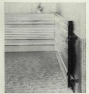
**Radiant heating panel** is 10" high and only 5%" thick. Camboard has a steel facing over two ½" copper tubes. Supply and return lines are coated with black mastic for heat retention. Cameron Thermodyne, Richmond, Va. For details, check No. 5 on p. 182
