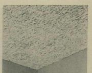
Acoustical tile has a textured surface that conceals joints, absorbs up to 90% of noise reaching it and reflects more than 70% of light striking it. Acoustone Glacier comes in 12"x12" and 12"x 24" tile with plain or foil backing. U.S. Gypsum, Chicago. For details, check No. 23 on p. 182
