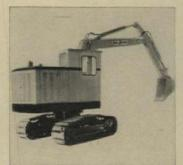
**Hydraulic backhoe** with  $\frac{1}{2}$ -yd. capacity is mounted on an Insley crawler. The C-10 weighs 23,890 lb., has a forward reach of 24'7" from kingpin, can dig 15'8" deep, undercut a slab by 7'5", dump a full load at 14'5". Hein-Werner Corp., Waukesha, Wis. For details, check No. 34 on p. 182
