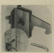
**Component hook** for joining panels with skins on both sides has a concealed action lock operated by a special wrench. It is available for panels with t&g or butt joints. Hook can withstand a 2,000-lb. pull. National Lock Co., Rockford. Ill. For details, check No. 9 on p. 182
