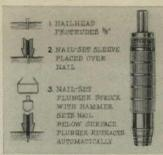
Nail set centers automatically and sinks nail into wood without marring its surface. 1. Nail is driven in so it protrudes 1/8". 2. Nail set is placed over nail head. 3. Hammer blow sets nail below wood surface. Stanley, New Britain, Conn. For details, check No. 15 on p. 182
