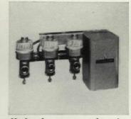
**Hydronic zone valve** has power supply, switching relay to cycle the circulator and heating plant, terminal block to join the wiring system, and two to four valves on a compact manifolding. Valves have only one moving part. Hydrotherm, Northvale, N.J. For details, check No. 3 on p. 182
