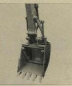
**24" backhoe bucket** is designed for use in sticky soils. A U-shaped blade scrapes the inside of the bucket to assure complete dumping. Unit can be supplied with new equipment or for existing machines. Deere & Co., Moline, Ill.
