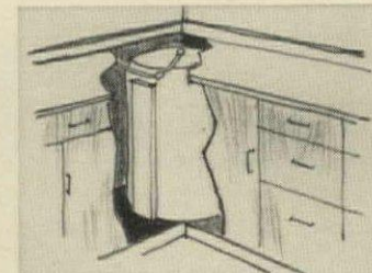
WATER HEATER fits under a hard-to-use counter corner and lets the existing water heater serve an added bathroom.
