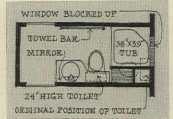
BATH ONLY 4½' WIDE gains storage space with square tub, gains counter space with the vanity extended over the toilet.
