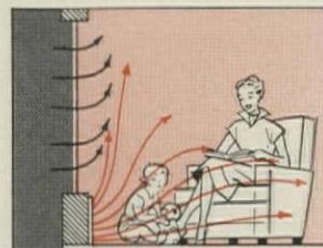
When walls and floor are warm, cold drafts are eliminated—all the space in the room is comfortably warm.
