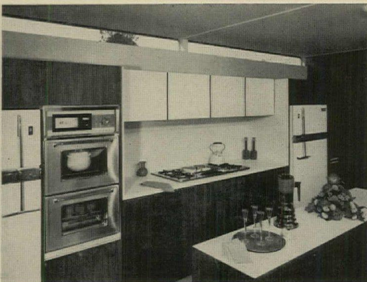
KITCHEN (B) has countertops and backsplashes of mosaic tile, cabinet facings of white laminate and walnut veneer. Food preparation island, at right, is on casters, can be rolled to any part of the room.
