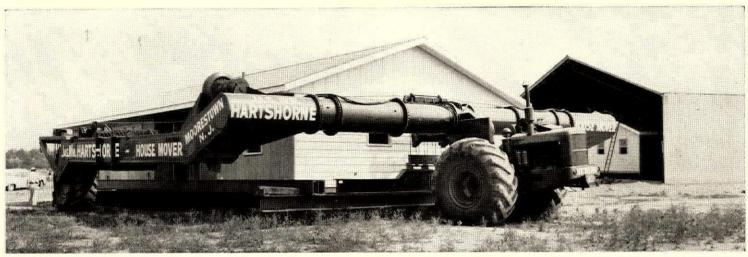
HOUSEMOVER is 100-ton yoke and tractor with 8' wheels. It carries house on steel cross beams at front and back. This 1,100 sq ft house sells for \$14,000.
