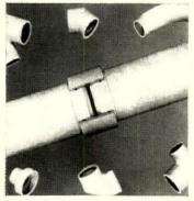
Sewer pipe of asbestos-cement is available with crush strengths of 1500 or 2400 lbs per lineal foot, 4" and 6" diameters. System includes rubber gasketed fittings. Certain-teed Products Corp. Ardmore, Pa.
