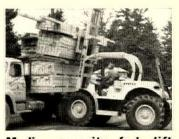
**Medium-capacity fork lift** handles up to 12,000 lbs, has four-wheel drive designed for jobsite lumber handling. It can tow loaded trailers, or can itself be towed to the site with drive disengaged. Hyster Co., Portland, Ore. *For details, check No. 158 on p 219*
