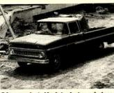
**Chevrolet light-duty pickup** has new 140-hp six-cylinder engine, is also available with heavy duty 165-hp engine, or 175-hp V8 engine. Trucks feature independent suspension system. Chevrolet Motor Div., Detroit.
