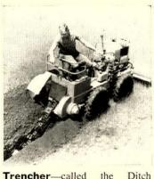
Witch—has pivoted front axle, can be steered for directional trenching. Standard unit can dig up to 12 fpm, or, with high-speed sprocket, up to 17 fpm. Charles Machine Works, Perry, Okla. For details, check No. 155 on p 219
