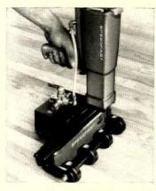
Automatic stapler has attachment which spaces staples and fires fastenings as tool is rolled along surface. Spacing can be from 2" to 8". Gun uses staples or nails from 5%" to 2". Speedfast Corp., Long Island City. For details, check No. 171 on p 219
