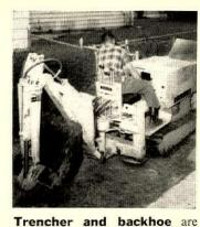
mounted on this crawler unit. Trencher makes cuts to 18" wide and 78" deep; backhoe has buckets up to 36" wide. Entire machine is only 37" wide. Davis, Mfg., Inc., Wichita, Kan. For details, check No. 154 on p 219
