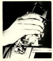
**Veneer trimmer** has swivel base which swings 45° in either direction, permits edge beveling of angled joints. Tool also scribes work and cuts it in a single operation. Stanley Works, New Britain, Conn.
