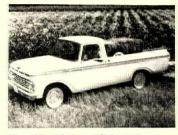
Ford half-ton pickup has new fully synchronized three-speed transmission, is available with integral or separate cab-and-box body, and with metal or wooden box floor. Ford Motor Co., Dearborn, Mich.
