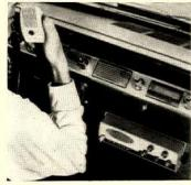
Two-way radio is an all-transistor 5-watt citizens-band transceiver operating on a.c. or d.c. Cadre 510 has a 20-mile range, is 113/8" x 33/8" x 53/8", weighs 6 lb. Brushed aluminum and charcoal finish. Price \$199.95. Cadre Industries, Endicott, N.Y. For details, check No. 19, p 162
