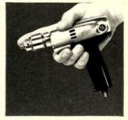
Compact 1/4" electric drill is 61/2" long, 2" at widest part, weighs 27 oz., runs at 1,250 rpm on 115-volt a.c. Diode converts input to d.c. and permits compact d.c. motor which supplies full power. List price: \$32.50. Thor Power Tool, Aurora, Ill.
