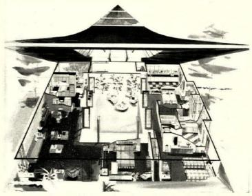
**CUTAWAY** with roof tilted up shows how the living-dining-kitchen wing (at left) and the bedroom wing (right) enclose an open atrium.
