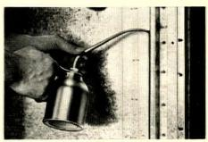
**Duct sealer** for high-pressure systems can be applied by brush, caulking gun, or pressure extruding equipment. It skins over in five to ten minutes, is tack free in an hour, and reaches maximum hardness in one to three days. The sealer fills voids up to ½" thick, withstands pressures up to 5psi. One gallon will extrude about 375' of ½" bead. Minnesota Mining & Manufacturing, St. Paul.
