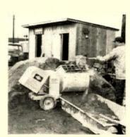
**Utility mixer** has 6 to 8 cu. ft. capacity for contractors who occasionally do big-volume work but do not need a heavy-duty mixer of this capacity. It is available with gas or optional electric drive. \$495 f.o.b. manufacturer's plant. Muller Machinery Co., Metchen, N.J.
