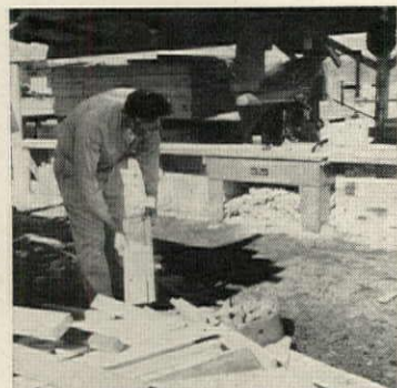
SALVAGE CUTTER makes blocking, cripples, and other small pieces from component cutter scrap and production line rejects.
