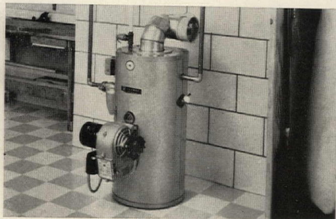
OIL-FIRED BOILER comes in 72,000 and 90,000 Btuh models. Units stand 35 \frac{1}{4} " and 38 \frac{1}{4} " high, are designed to fit in a 2'x3' space. The combustion chamber is made of a new precast ceramic material, and a light-sensing cell housed in the cool end of the burner instantly reacts to ignition and shutdown.
