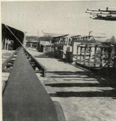
PRECUT LUMBER CONVEYOR runs almost entire length of factory, delivers pieces to storage bins for component assembly operations.
