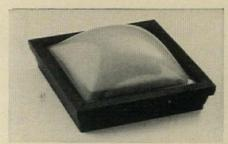
Insulating skylight has dead air space between inner and outer domes to reduce heat loss. Domes come in clear acrylic and three shades of white. Frame is made of tough PVC (polyvinyl chloride) plastic—a poor heat conductor—to reduce heat loss and condensation. Corrulux Double-domes are completely factory assembled.
