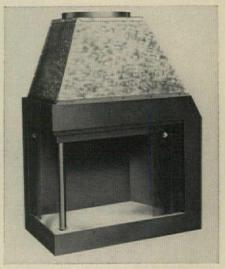
Prefabicated corner fireplace needs no mortar or masonry. Left- or righthand models are made for either flushto-floor or raised-hearth installation. Unit is engineered with inner air circulation between shells so it can be safely butted against combustible surfaces.
