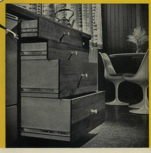
No. 1300. For loads to 50 pounds. Only ½" clearance required each side. Nylon ball bearing wheels for noiseless, smooth lifetime operation. Economical, easy to install. Bright zinc-plated finish. Sizes from 12" to 28". Most widely used drawer slide on the market.
