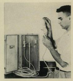
Water level consists of a pair of sighting instruments connected by a long flexible plastic tube. It is marked with graduations of 0.001" with a range of up to 6". It is used for checking level (or measuring differences in height) in foundations, grading; can be used where transit sight line is obstructed.
