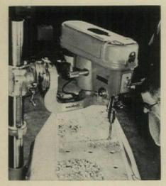
**Drill press** saves time because the tool moves over the work and eliminates the need for exact positioning of the work on the table. With Unidrill the operator can move the cutting tool up and down, 360° around the column, and in and out from the column, or tilt the head as much as 45° left or right.
