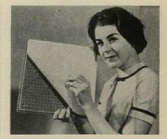
Washable ceiling is made possible by a thin film of embossed vinyl stretched across perforations of wood fiber tile. Noise reduction coefficient in the 250 to 2,000 cps range is 65, better than many other acoustical tiles. Tiles are installed like any ceiling tile, come in three patterns: embossed white, heavily embossed white, embossed sandalwood. Price: 33¢ to 35¢ retail.
