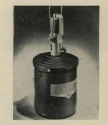
Small airless pump to cut overspray in medium production will handle all conventional paints with a standard airless gun and a compressor as small as 1 hp. Pressure is supplied by a chromium piston in a stainless steel cylinder, operated by an air motor. Price: \$192.50 FOB Toledo. DeVilbiss Co, Toledo.
