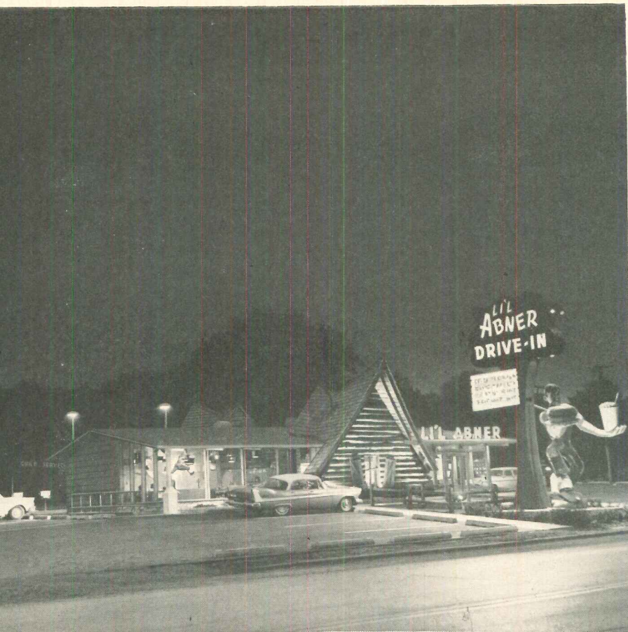
Approaches and service area of Li'l Abner Drive-In, Morton Grove, Ill., are well lighted by 18 L-M Post Top Luminaires. PTL's are available for mercury or incandescent, with choice of seven IES light patterns; with photocontrol if desired.
