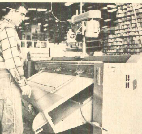
DOOR MACHINE turns out ready-hung doors. One man can assemble 100 doors in a day.
