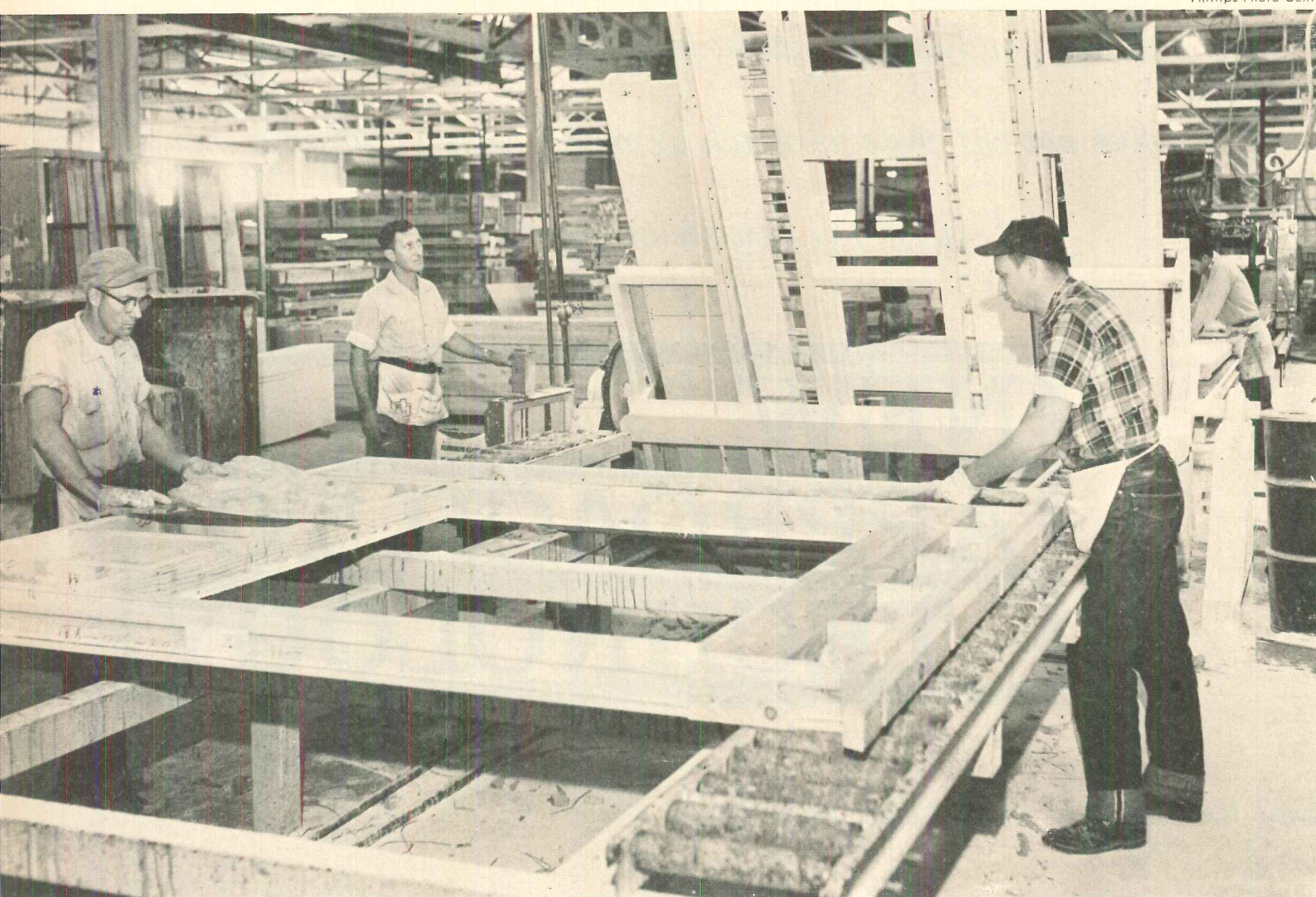
IN-PLANT LABOR can produce more with help of efficient production machinery. This is production line at National Homes' Lafayette plant.
