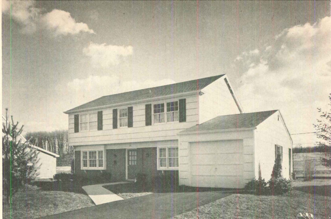
New two-story (plan at left) has 1,854 sq ft—100 sq ft more than previous version (plan at top). In new model, stairs and powder room were relocated to provide true center hall, family room was enlarged by extending part of kitchen into laundry area behind garage. Four-bedroom house has trim garrison front (second-story windows align with first-floor door and windows), sells for $17,500 with air conditioning and 8,400 sq ft lot. Three-bedroom version (right) has 1,772 sq ft and same first-floor plan, sells for $16,990.
