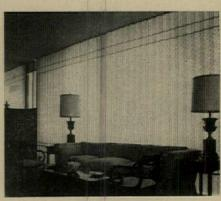
Traversing drapes are made of small squares of rigid plastic. Small slots in molded sections admit air. Light and heat are controlled by traversing drape or by a choice of opaque or translucent colors. Heat transfer is claimed to be 1/1000 that of aluminum. New drape stacks one foot to the inch, ie, a 10' drape stacks in 10"
