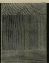
DOUGLAS FIR—tough, straight-grained wood for interior trim, millwork, and applications requiring stiffness and nailholding power. In stress grades, it offers exceptional strength for framing.
