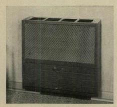
Coleman now offers a through-the-wall gas heater with a sealed combustion chamber. Two models give 22,000 and 30,000 Btuh from case 30"x26"x9". Unit fastens to studs 434" above floor. Outside air is used for combustion and exhaust vents directly to outdoors. Options include manual, automatic, or remote controls, two-speed blower, vent extension for thick walls, decorative insert panels.
