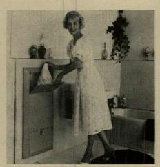
Built-in hamper takes no floor space, can be concealed behind a door or in a closet. Capacity is more than two washer loads. Heavy guage steel will not absorb odors. Vents top and bottom allow free air circulation. Price, about the same as wall tile it replaces.
