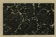
flooring is offered in latest Hydrocord-backed Vinyl Corlon. Palatial is a marbleized pattern with veins of clear and translucent vinyl in a textured field of ground vinyl particles. It has, the company claims, the finest maintenance characteristics of any flooring Armstrong makes. Cost: about \$1.10 a sq ft installed.
