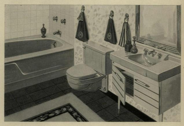
You can give such tenant-pleasing extras if your bathroom plans are economical. Cut costs by aligning three fixtures on one wall—save still more by placing the toilet between tub and lavatory.
