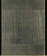
WHITE FIR—strong and lightweight for framing, roof decking, paneling and moulding, it is easy to cut, saw and shape. Popular, too, for interior and exterior trim and many industrial uses.
