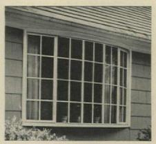
Complete casement bow is made as one unit. All joints are dovetailed for strength, weathertightness, and narrow mullion lines. Top and bottom casing are shaped to bow radius, glued and screwed to head and seat. All wood is Woodlife treated. Hardware includes extension hinges, roto gears, cam-action locks. Screens are alodized aluminum.
