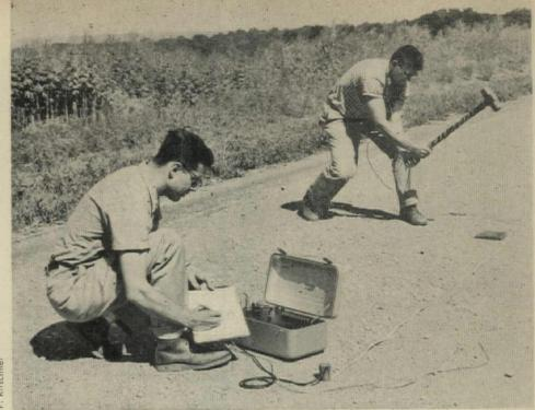
SEISMOGRAPH reveals rock's hardness and depth by analyzing shock waves set off by hammer blow.
