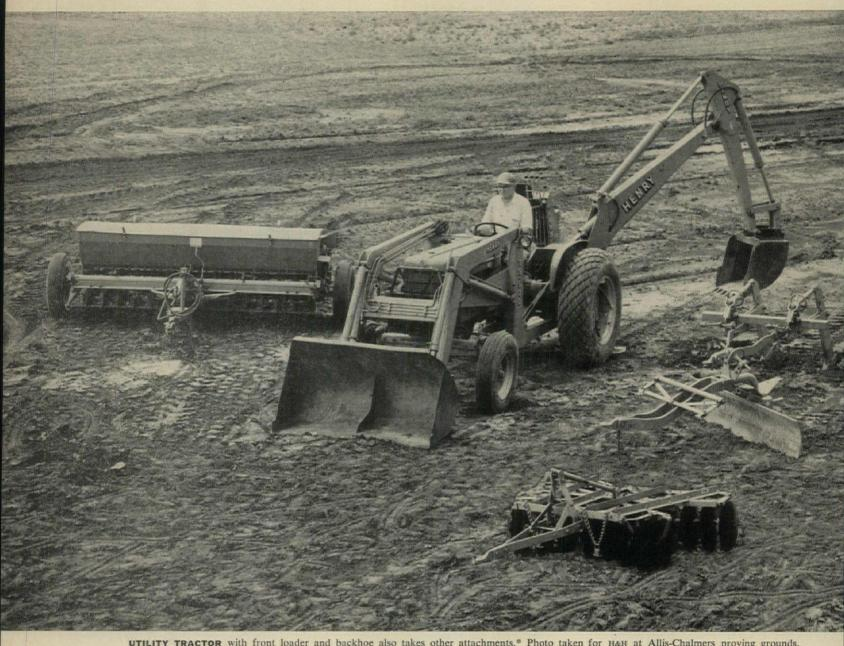
UTILITY TRACTOR with front loader and backhoe also takes other attachments.\* Photo taken for H&H at Allis-Chalmers proving grounds.
