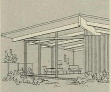
Ridge beams and exposed ceiling 'beams of fir plywood are smooth and attractive. Longspan beams make sense in home building because they permit maximum design freedom.
