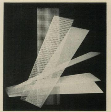
**Plastic louvers** give a high-intensity but well diffused light from overall ceiling fixtures. Mystic Gratelite comes in two panel sizes: 11''x48'', 16''x48''. Cubes are  $\frac{3}{8}''$  on a side, but polystyrene is translucent so panel looks solid. Gratelite hides tubes but allows free interchange of air. It can be easily cleaned and destaticized by a dip in detergent.
