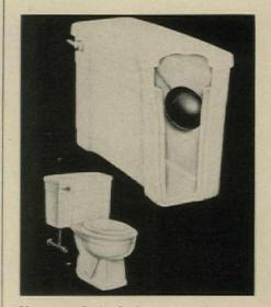
Non-sweat tank is now optional on most Universal-Rundle Uni-Closets. The tank is insulated with a foamed polystyrene liner to keep the water from chilling the shell, causing condensation. Tank comes in white and all U-R colors, needs no special fittings for installation. Ever-Dry was field-tested for five years. Universal-Rundle, New Castle, Pa.
