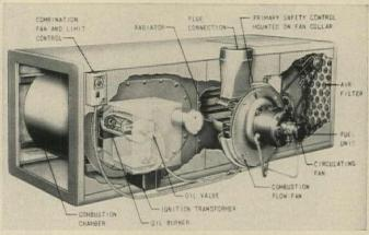
**HOW IT WORKS:** combustion flow fan on flue side insures complete fuel and air mixture, cools exhaust as it blows it out.
