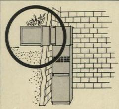
**4** The cooling unit is inserted into the sleeve, anchor brackets attached, seams caulked and electrical connections made. There are no refrigerant lines, no plumbing, no specialized on-the-job construction, no installation delays.
