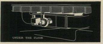
UNDERFLOOR UNIT can be vented through basement wall.
