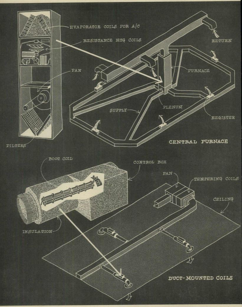
TWO BASIC SYSTEMS for electric warm-air heat-central furnace or room heaters in ducts-can be used with ducts either in slab (or crawl space) or overhead.
