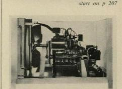
Air cooling by gas uses natural or Lp fuel to power a Continental engine. In this system by Gas-cool, models of 5-ton and  $7\frac{1}{2}$ -ton capacities are claimed to operate up to 60% cheaper than all-electric models. Fuel consumption is only 20 cu ft of 1,000 Btu natural gas per ton-hour. Five-ton model rates at 60,000 Btuh, bigger model at 90,000 Btuh. Vector Engr Contractors, Dallas.
