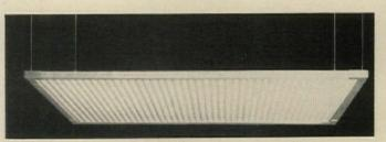
**Island of light** is supplied by suspended plastic grille of Diffusa-Lite's unit luminous ceilings. Vinylux plastic panels have concave and convex surfaces that eliminate glare and contrasts. Diffusa-Lite panels come in eight sizes: from 3'x'4 to 6'x9'. Vinylux plastic comes in 18'', 24'', and 36'' wide rolls. Two-light fluorescent fixtures are available to match diffusers.
