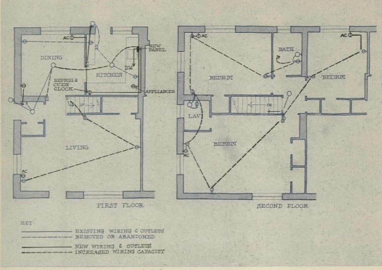
**REWIRING** adds kitchen appliance outlets and separate circuits for refrigerators and dishwashers. Air conditioning outlets will be installed in every major room but tenants must supply own units.
