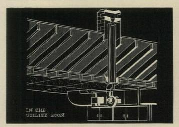
UTILITY ROOM UNIT above cabinets vents through prefab chimney.
