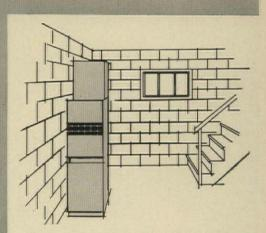
**2** In the Thermo-Center, the unit is moved to an outside wall. There's no change in the amount of ductwork required, nor is the system operation affected in any way. Heating units can be upflow, downflow or horizontal; gas or oil.
