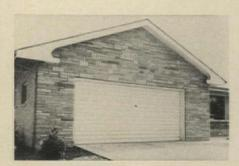
**Lightweight door**—the Raylon—combines aluminum frame with translucent fiberglass-reinforced panels. Door is claimed to be immune to corrosion, warping, shrinking, splintering. It comes in green, tan, and white, in standard sizes, 8'x6'6" to 16'x7'. Normal headroom is 12", reducible to 3" with Raynor Converti-Kit. One-year guarantee.
