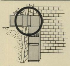
**3** Next, the prefabricated sleeve and transition assembly is built into the wall and joined to the furnace plenum and ductwork. The sleeve and transition assembly can be applied to any type of wall construction – frame, brick or concrete.
