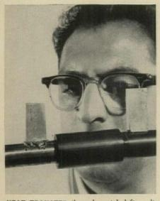
HEAT TRANSFER through metal, left, melts test alloy, which stays solid on Geon, right.
