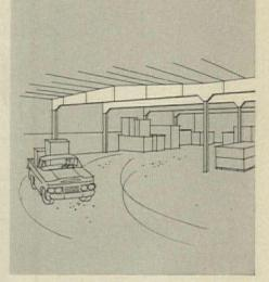
This warehouse illustrates use of low-cost, strong plywood beams to create a 40' x 80' clear area free of supporting posts or walls. Four peaked beams, spaced 20 ft. o.c., span 40 ft.
