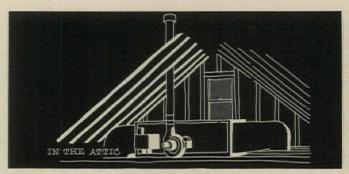
ATTIC UNIT needs only a stub flue through the roof.
