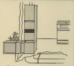
**6** In a house built on a slab, the transition is joined to a Thermo-Center downflow plenum which supports the Winter Weathermaker. The plenum directs air from the heating and cooling units into the duct system.
