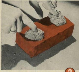
The mortar that stays plastic longer will be the one having the highest water retention. Notice the greater plasticity of the Brixment mortar!
