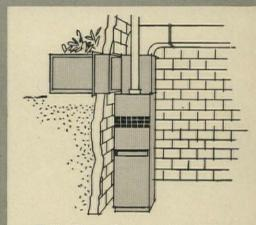
**5** The Thermo-Center can be applied to any type of home – ranch, split level or multi-story. In a house with a basement, for example, the cooling unit is connected to a plenum set on top of an upflow Carrier Winter Weathermaker.
