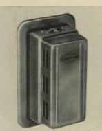
**Humidistat** by Kitchen-aire controls moisture content of air by operating ventilating fans in bath, laundry, kitchen. Control uses a 150-strand human-hair element to activate unit for any setting between 10% and 100% relative humidity. New unit is single-pole, double-throw, lineor low-voltage, a-c or d-c.
