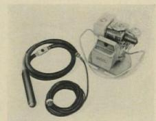
**Self-powered vibrator** combines an 80-lb, 1200-w generator with a 25%" diameter vibrating head. The new head reverses usual practice, has an outside rotor and inside stator. Eccentric rotor is the only moving part. Generator armature whirls in air, held away from other parts by magnetic field.
