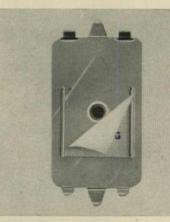
**Easy-to-find outlet** is assured by new outlet covers for use in plaster walls. When outlet box is installed, it is covered with the new device and protective tape is peeled off. When box is plastered over, a dye in the cover plate seeps out and shows through the plaster to locate the box. When cover is broken out, it leaves a clean hole.
