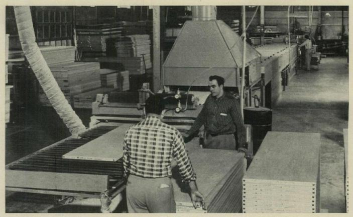
SURFACER carries plywood through friction rollers, roller coater, drying oven, and two more sets of friction rollers.
