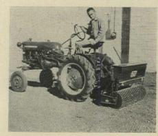
**Roller blade** will level 600 sq yd of rough graded area in 20 minutes simply by driving over it. With a seed dispenser it will seed, fertilize, cover, and compact the same area in ten minutes. Blade floats behind wheels, shears soil to desired level; mesh roller follows blade, pulverizes, mulches, and compacts soil. Unit come 4' and 6' wide.
