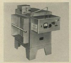
**New electronic filters** from Electro-Air are less bulky and less expensive. The new units (there's one in the Universal line, two each in the Tec and Compact lines) have reduced cell spacing (to 5/16") and redesigned cell and power pack, but keep basic system used in high capacity commercial and industrial equipment. New models keep 90% efficiency rating.
