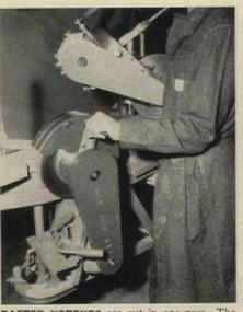
**RAFTER NOTCHES** are cut in one pass. The manufacturer claims all cuts are so precise, repeated parts are fully interchangeable.
