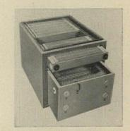
York's new electronic filters come in three model series—120, 160, and 240 sized 22" x 20" x 21", 22" x 24" x 26", 22" x 24" x 29". Largest size handles 2,400 cfm, has about 14,000 sq in. of collecting plate area. York filter units are designed to be installed in ductwork, have drawertype plate sections which are easily removed for cleaning. York Div, Borg-Warner, York, Pa.
