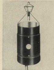
Post lantern switch turns yard lights on and off at dusk and dawn. Time-delay photoelectric eye activates switch, allows three-minute lag so lights will not be turned off accidentally by car headlights. Unit is compact, prewired, will fit any 3" post. Switch works on 115v with 400-w capacity. Temperature compensator will withstand -25F to 150F.
