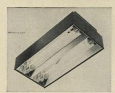
**Quartz infra-red heater** develops filament temperatures of up to 4,000F, is particularly adapted to outside use since its radiant energy will not be dissipated by cold air and it is not affected by moisture, atmospheric changes, etc. Luminator units come in one-lamp fixtures of 500 w to three-lamp furnaces of 15,000 w.
