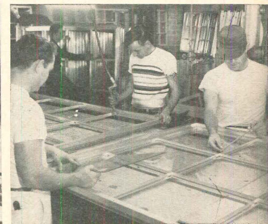
12 Aluminum windows, purchased outside, are glazed in the plant. First a moisture-proof seating compound is air-gun applied, then the glass fitted in place. Finally, neoprene strips seal in glass.
