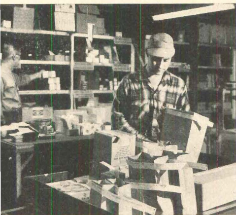
28 Cartons of miscellaneous materials (calking compound, nails, bolts, screws, etc) are carefully packed. Each has IBM identification number to make sure package is complete.
