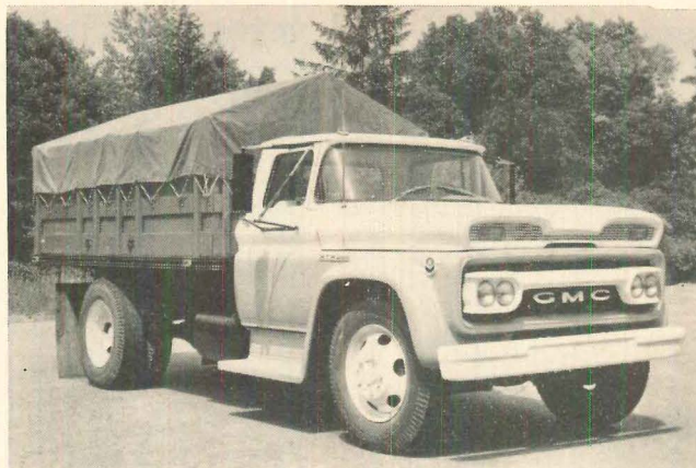
V-4000 STAKE TRUCK is 105" from bumper to back of cab.
