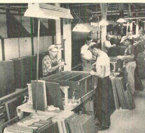
25 Cabinets are assembled at 650-a-day rate on this line. This process includes hanging the doors, attaching magnetic hardware, inserting plastic drawers, and adding the door pulls.
