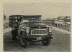
B-160 STAKE TRUCK can have 129" to 189" wheelbase, 154-hp six, 154.8-or 193.1-hp V-8.
