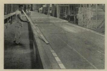
PATTERN STRIPS ARE INSERTED in slots in framing table. Top and bottom strips are color coded (pink and blue) to avoid mistakes.
