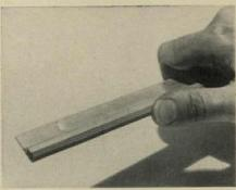
New vinyl weatherstrip is made to insulate against drafts, sound, light, and dust. An aluminum strip holds a vinyl insert with four continuous ridges. Strips are ready mitered, have screw slots to adjust fit to jamb and door. There are no interlocking pieces to adjust. Vinyl insert will not become soft or sticky and will not "pick". The aluminum alloy takes paint well. Strips may be prepainted to match the jamb so the door can be used immediately.
