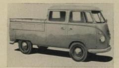
**Double-cab pickup** is latest version of the VW truck. Cab seats six as work crew carrier. Rear seat can be removed to give 63 cu ft of enlosed lockable space. Sides of 32-sq ft rear deck drop so it can be loaded from all sides. Body mounts on standard VW chassis. Price on east coast: \$2,150.
