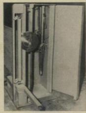
Door trimmer is latest shop fabricating tool-from Turn-A-Bore. Door is placed on edge in the trimmer. High-speed saw is moved smoothly across door end by a combination of air and hydraulic power to insure a smooth splinter-free edge. Machine will trim doors of any style.
